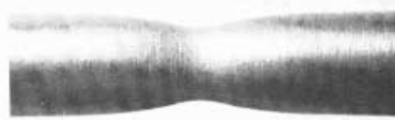
Figure 3.2 Necking in a tensile specimen [37].
