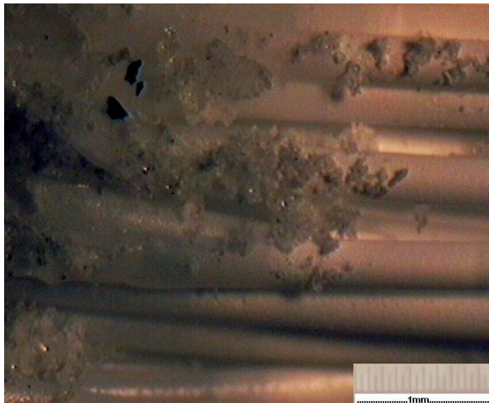
Figure 4.1.4 Lateral view of bundle configuration of virgin hollow fibers membrane.
