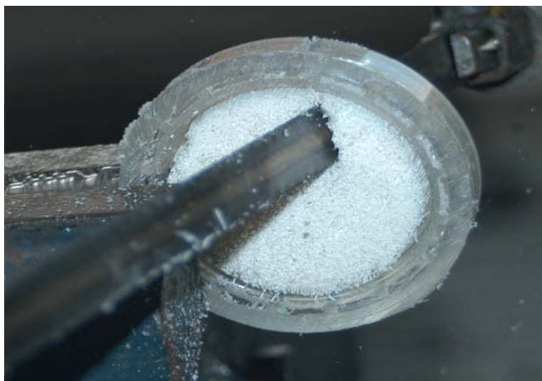
Figure 2.1.2 Cutting the upper part of the dialyzer into two parts.
