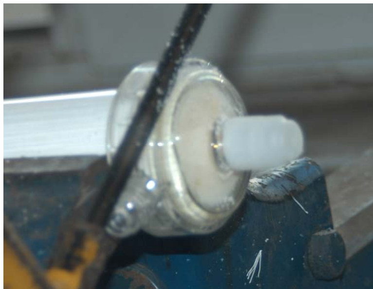
Figure 2.1.1 Cutting procedure of upper head of the dialyzer.
