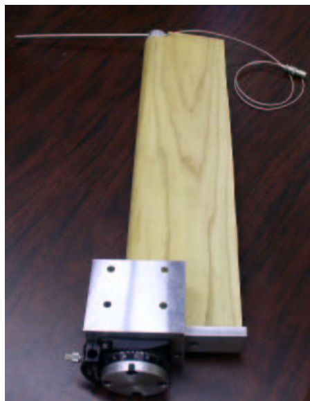
Figure 5: Sting design and angle controller that allows for angle calibration.
