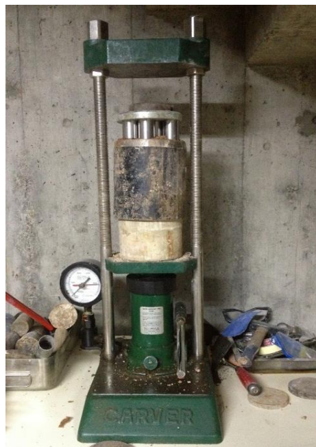
Figure 3.22 : Obtaining undisturbed soil samples by hydraulic jack.
