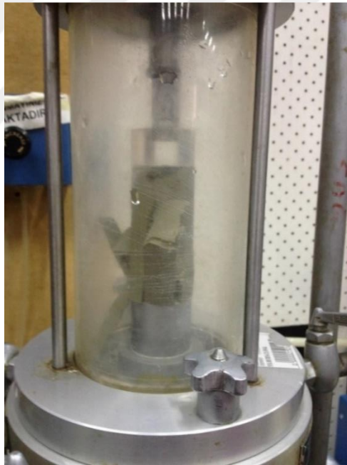
Figure 3.55 : A failed sample in unconfined compression test.
