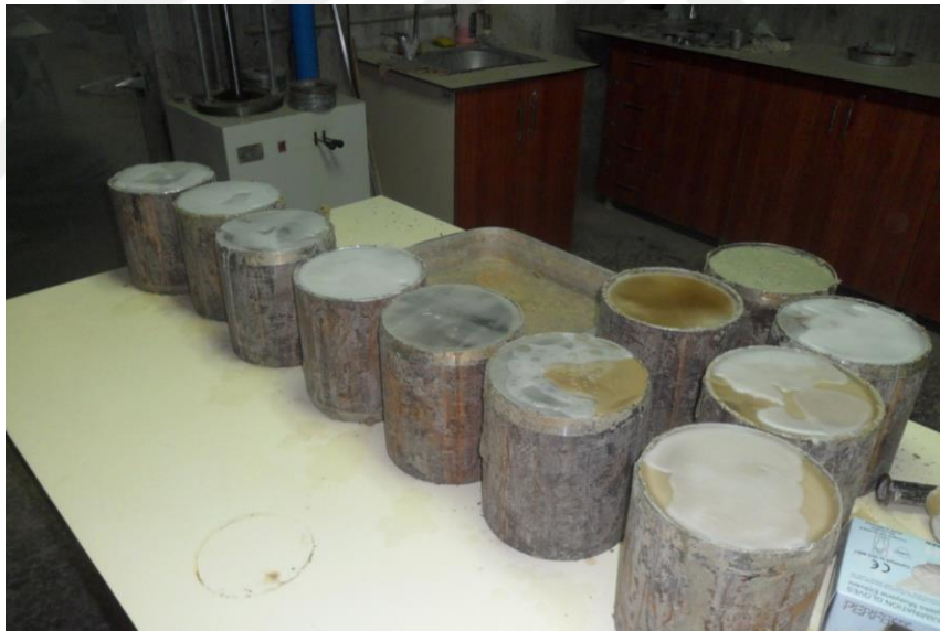
Figure 3.8 : Sample tubes sealed with wax.
