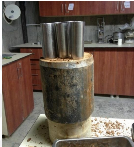
Figure 3.21 : Obtaining undisturbed soil samples for unconfined compression test.
