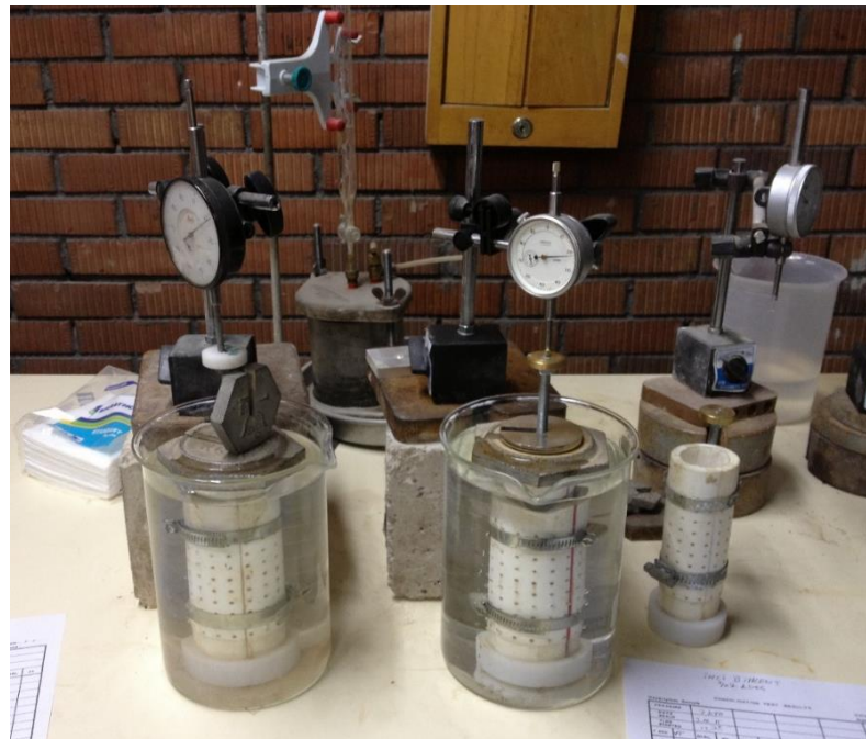
Figure 3.32 : Inundation process of the samples for unconfined compression test (soaked condition).
