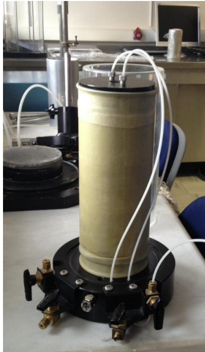
Figure 3.41 : Soil sample confined by the membrane for resilient modulus test.
