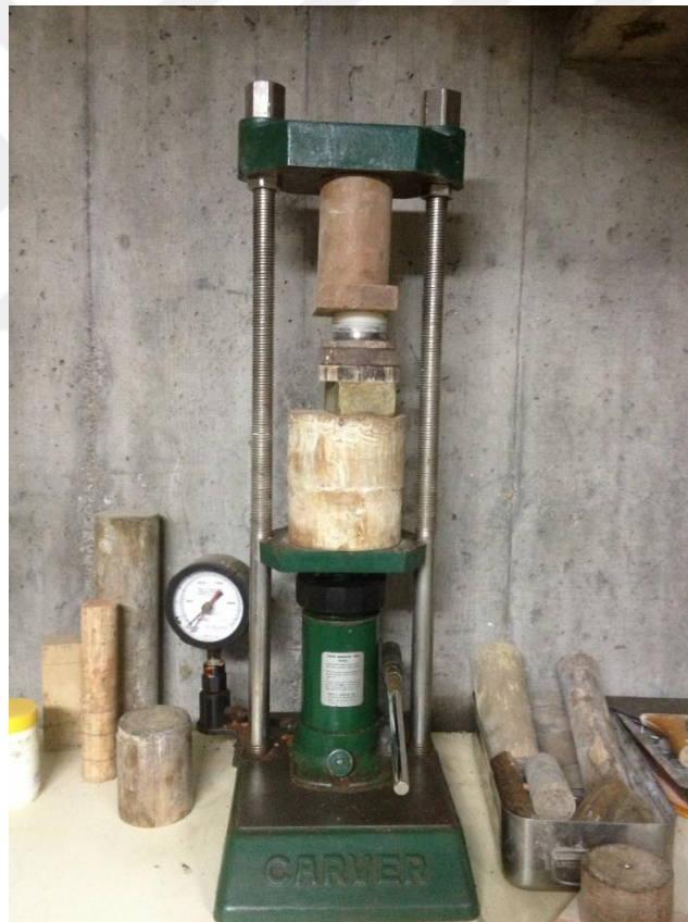
Figure 3.35 : Compaction of soil samples for oedometer tests.
