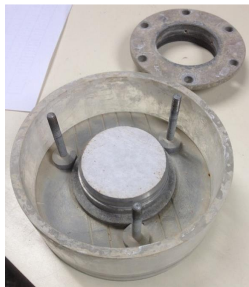
Figure 3.38 : Filter paper on the sample for oedometer tests.
