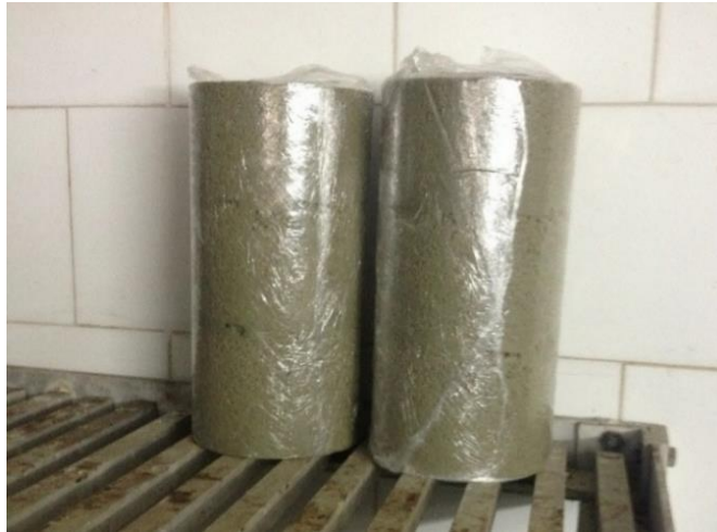
Figure 3.40 : Prepared soil samples of resilient modulus test for different cure periods in the moisture room.
