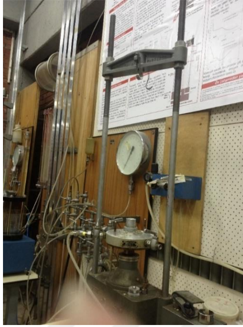
Figure 3.54 : Unconfined compression test loading frame.
