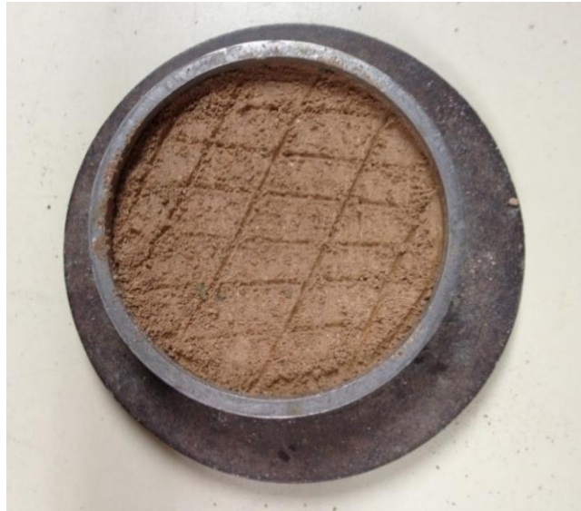
Figure 3.34 : Roughened soil samples for oedometer tests of Bilkent Clay.
