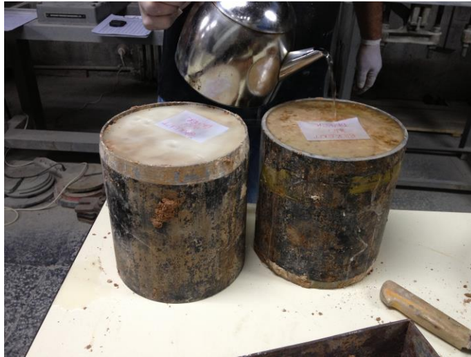
Figure 3.13 : Sealing of undisturbed soil samples with wax.
