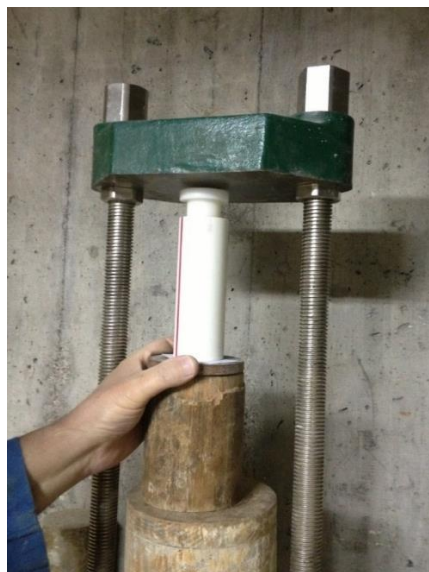
Figure 3.26 : Compaction process to get samples for unconfined compression test.
