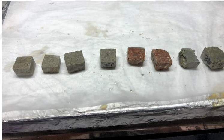
Figure 3.48 : Cube SEM samples.
