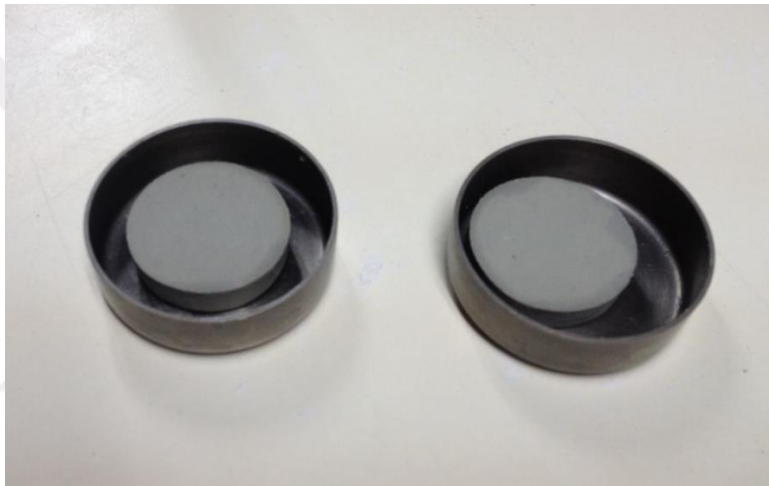
Figure 3.53 : Oven-dried soil sample of shrinkage limit test.
