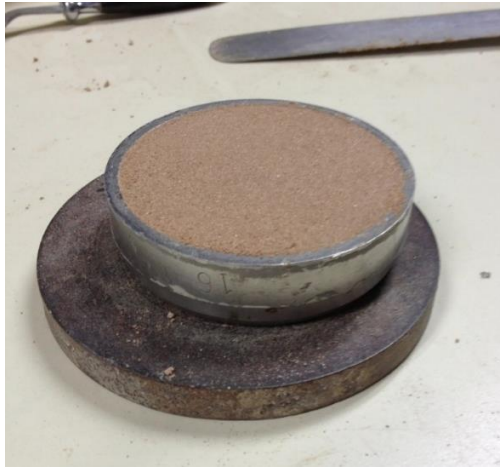
Figure 3.36 : Compacted soil sample in oedometer ring.
