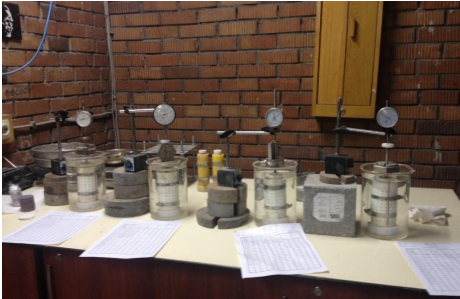
Figure 3.56 : Inundation process of the samples for unconfined compression test (soaked condition).
