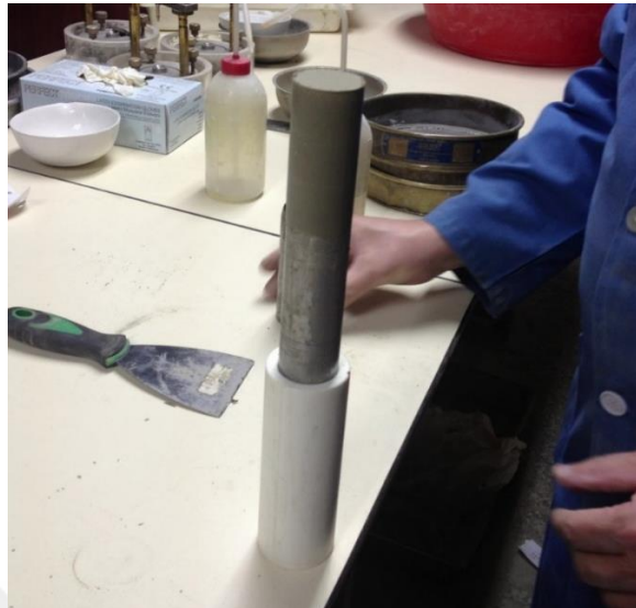
Figure 3.27 : Extracting of soil samples for unconfined compression test.
