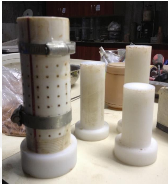
Figure 3.29 : Apparatus used for preparation of the samples for unconfined compression test (soaked condition).
