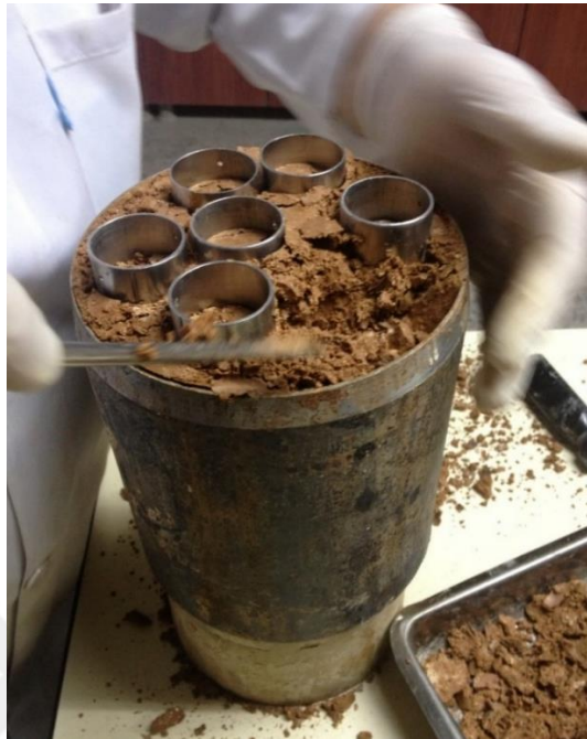
Figure 3.23 : Trimming process to get undisturbed soil samples.
