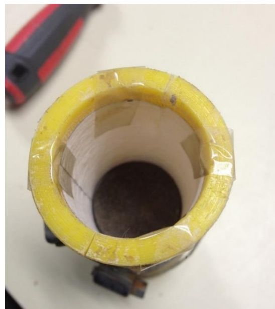
Figure 3.30 : The mould with filter paper for unconfined compression test (soaked condition).
