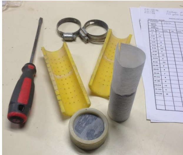
Figure 3.31 : Filter paper covering soil samples for unconfined compression test (soaked condition).
