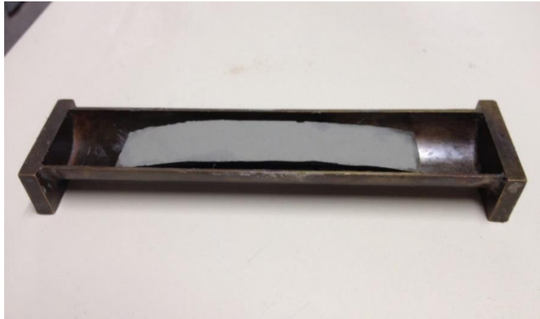
Figure 3.52 : Oven-dried soil sample of linear shrinkage limit test.
