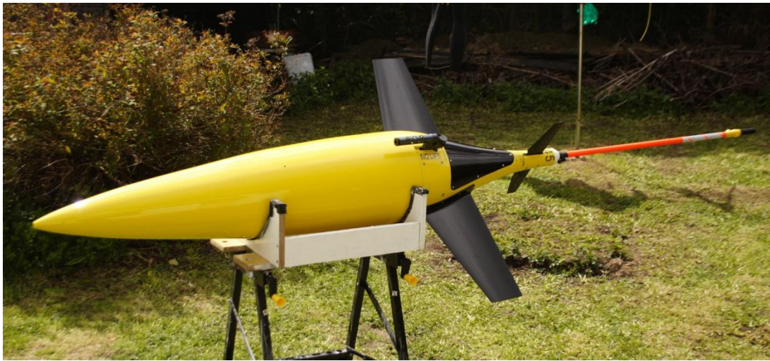
Figure 1.7 : Seaglider with its laminar flow body (Jones, n.d.).
