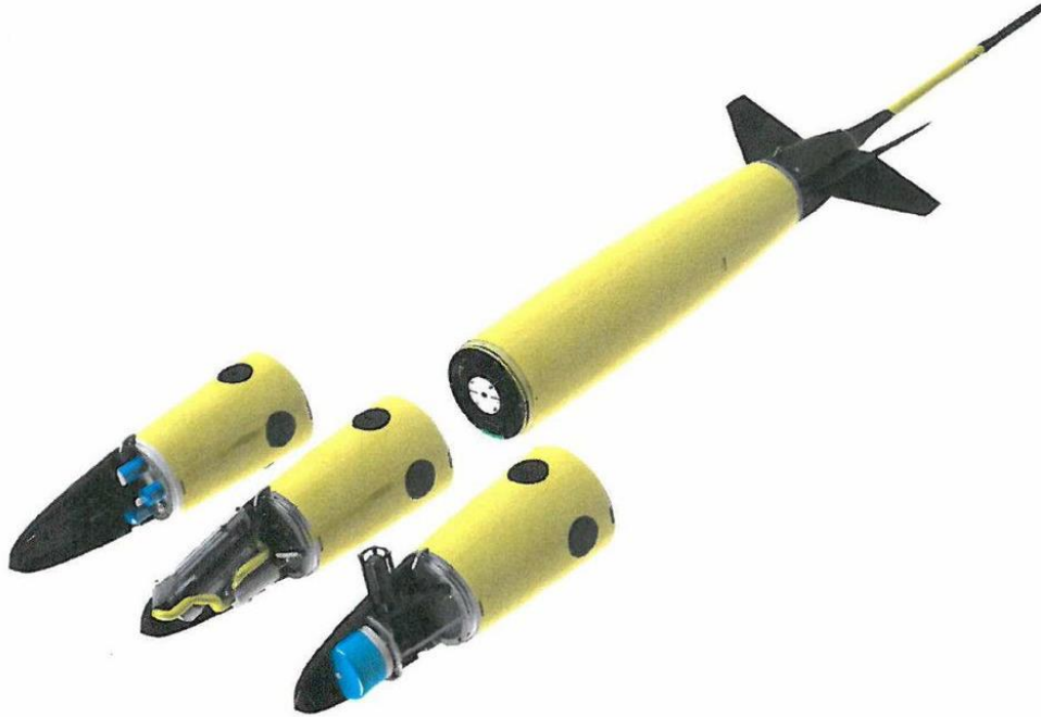
Figure 1.10 : A glider with modular science payload section (Szondy, 2015).
