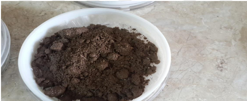
Figure 3.4. Petri dishes including 100gm soil sample use for extraction of nematodes in the Baermann method.
