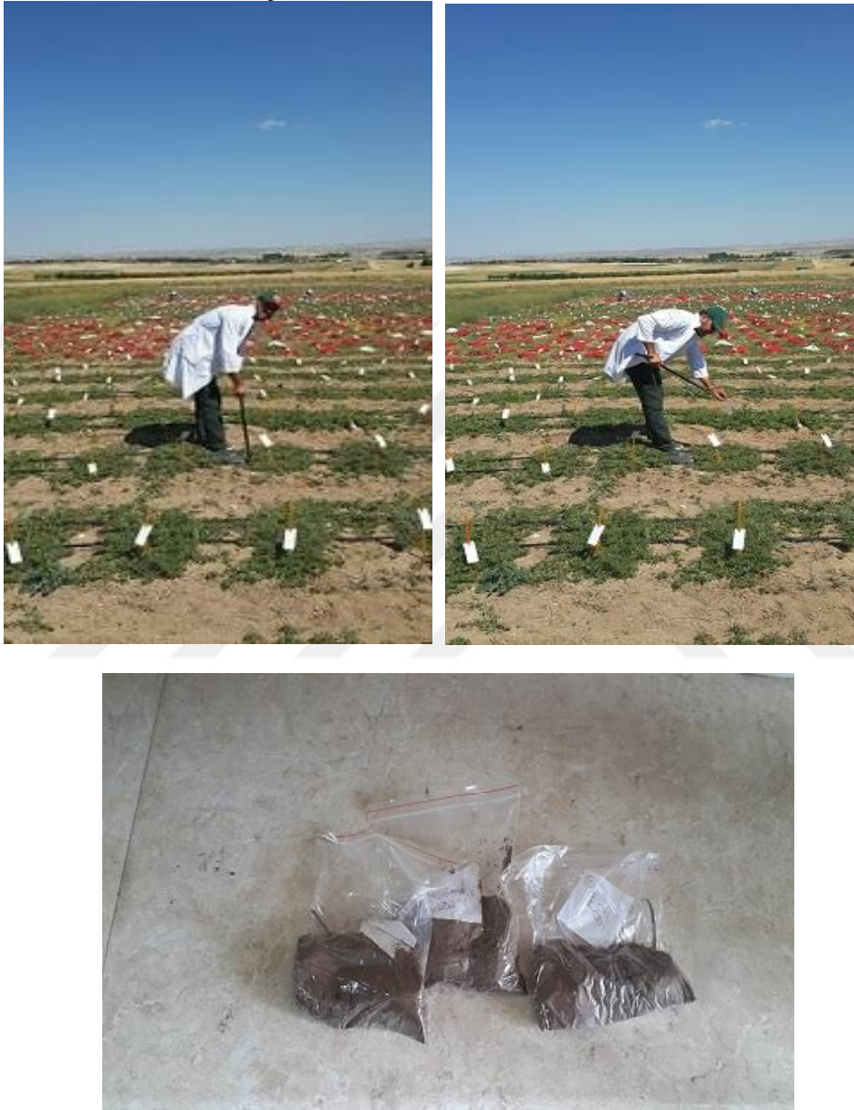
Figure 3.16. The sampling of soil by using soil Auger by 5 cm diameter in 10-20 cm soil depth.
