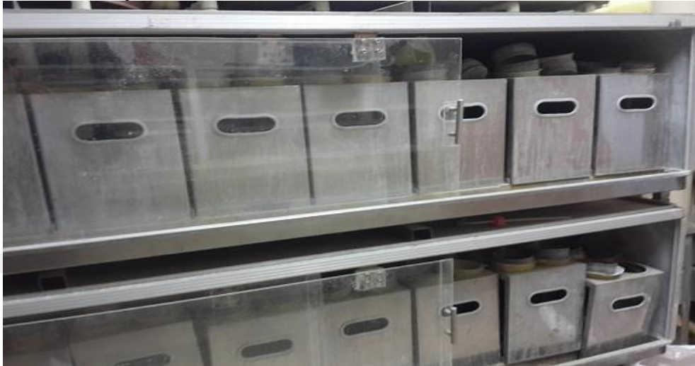
Figure 3.2. Misting chamber for the extraction of P. thornei , P. neglectus and D. dipsaci .
