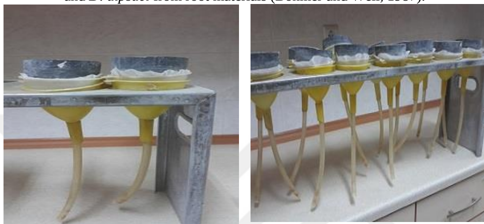
Figure 3.1. The Dubble funnel method for extraction RLN ( P. thorne , P. neglectus ) and D. dipsaci from root materials (Bohmer and Weil, 1987).
