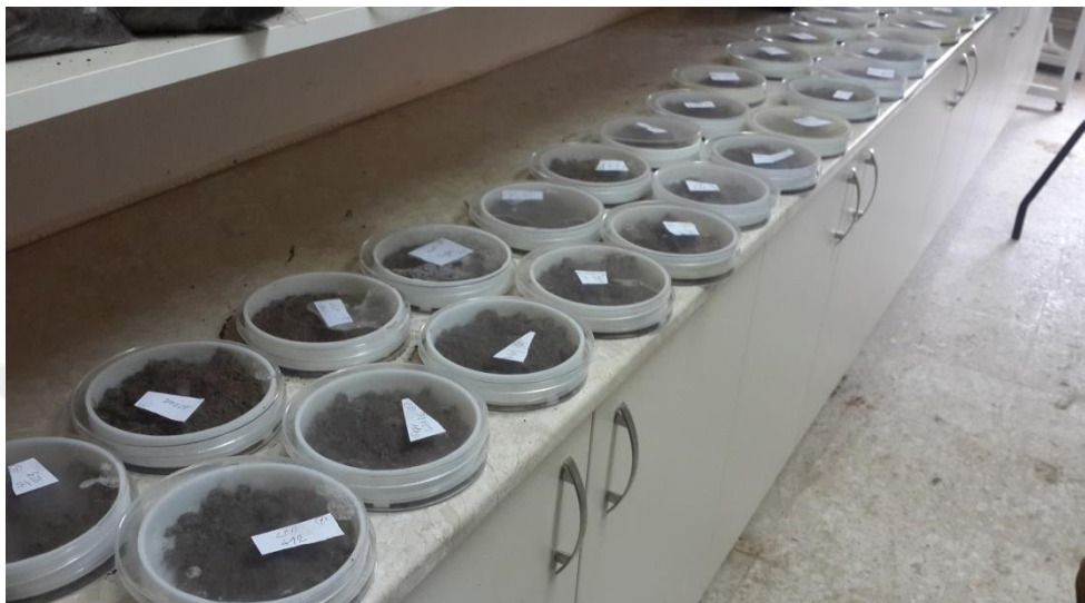
Figure 3.3. The Baermann method used the extraction of P. thornei , P. neglectus and D. dipsaci growing in the soil of chickpea fields and the plants themselves.
