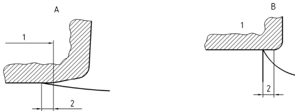
Figure 2.8 : Transition areas between journal and collar bearing surface – collar bearing surface and wheelset [12]
