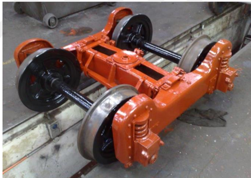
Figure 2.1 : The Fox type bogie developed in 1893 by Samson Fox
