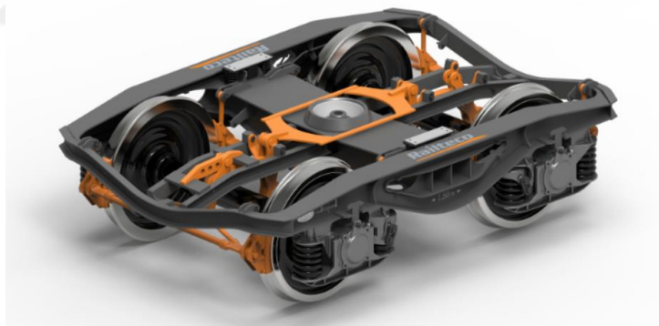
Figure 2.2 : Widely used today B-V category, Y25 type bogie
