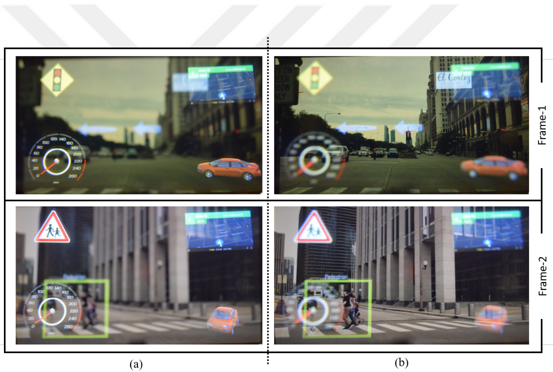
Figure 4.4: Experimental captures of the virtual scene. a) The camera is focused in 4 diopters (25 cm). b) The camera is focused in 2 diopters (50 cm). FOV is 60.0 by 35.5 degrees and the image can be seen with both eyes simultaneously.
