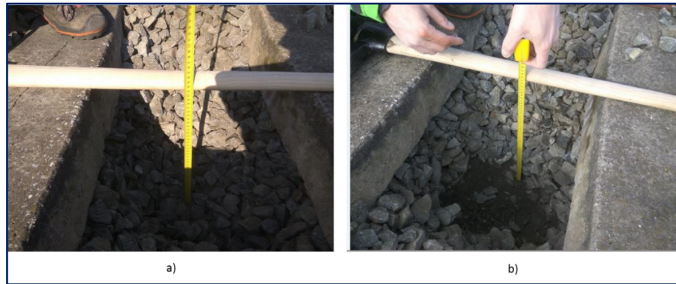
Figure 6.26. Trench 3: a) moderately clean ballast layer thicknesses measurement, b) moderately fouled ballast layer thicknesses measurement
