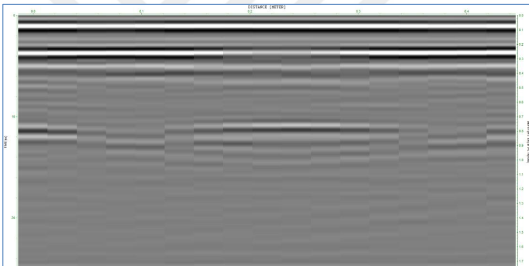
Figure 7.39. 1GHz antenna was used in transverse orientation in fouled ballast condition with two sleepers case: with 2 horizontal and 1 vertical steel rods imitating rail effect
