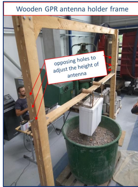
Figure 6.3. Wooden GPR antenna holder frame
