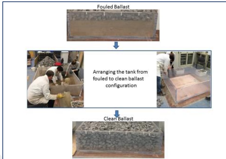
Figure 6.41. Fouled ballast configuration, the arrangement of the tank for clean ballast configuration and finally clean ballast configuration
