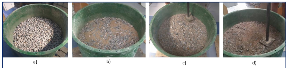
Figure 6.5. Configurations of a) clean b) sand-fouled c) fine gravel-fouled d) mixture-fouled finer granite ballast
