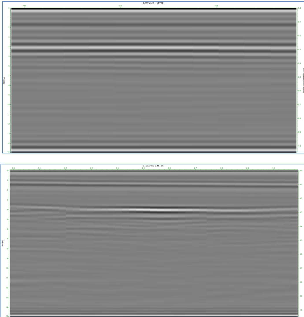
Figure 7.37. Comparison of radargrams from measurements with 2GHz NA antenna with 1 sleeper case in terms of longitudinal and transverse orientations in fouled ballast
