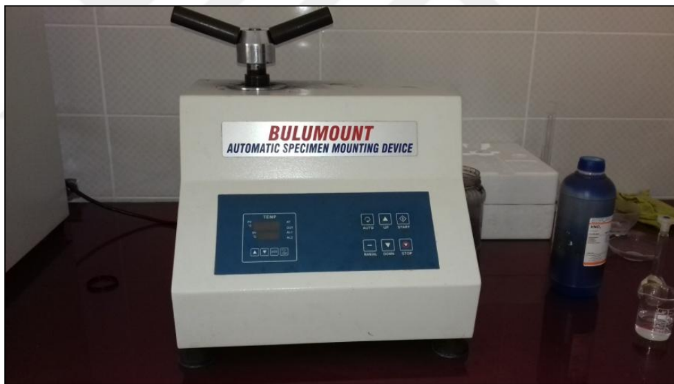
Figure 5.6. Machine used for mounting the specimens.
