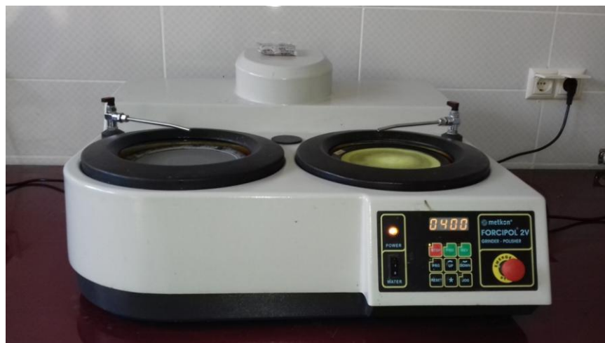
Figure 5.8. Machine used for grinding and polishing.
