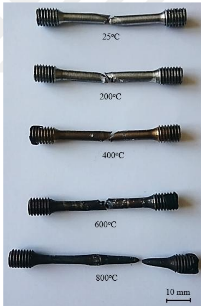
Figure 6.34 Failure mode of as-welded samples tensile tested at different temperatures.
