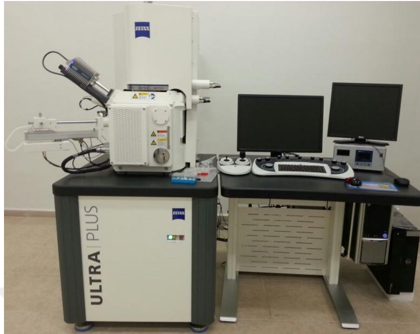
Figure 5.10. Scanning electron microscopy used in the present experimental work.
