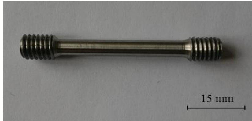
Figure 5.4. Tensile test specimen used for hot tensile test.
