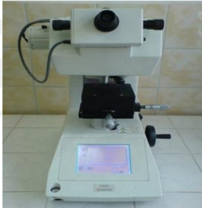
Figure 5.5. Shimadzu microhardness test machine used for the measurement of Vickers hardness.
