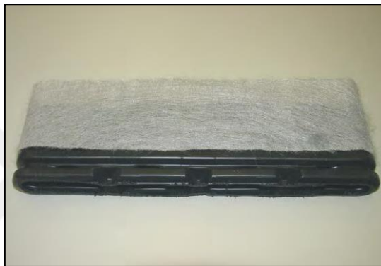
Figure 4.15 Geocomposite edge drain
