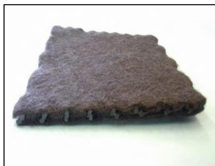
Figure 4.10 Geocomposite Geonet Drain
