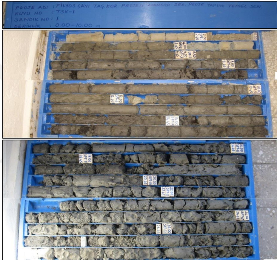
Figure 6.3 Sample drilling well of TSK-1 at 44.24 m
