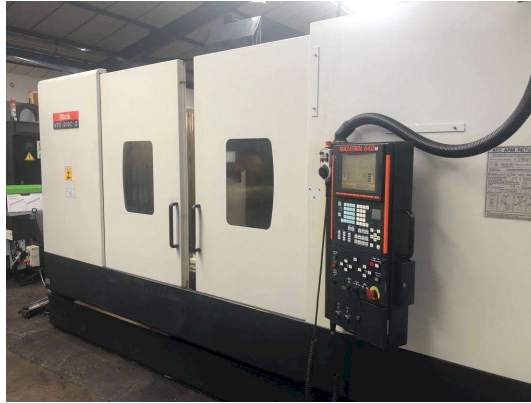
Figure 17. VTC-200C II / Yamazaki Mazak vertical machining device available in TOTOMAK company
