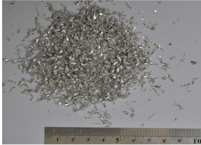
Figure 44. Chip forms of AZ91/2.5 wt.% rCF composite at conditions: V_c :560 m/min, V_f :0.95 mm/min
