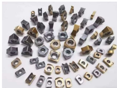
Figure 12. Types of face milling inserts 47
