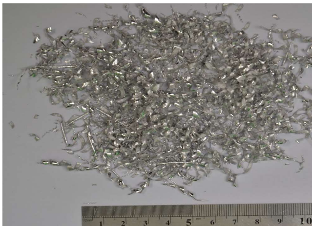
Figure 43. Chip forms of AZ91/2.5 wt.% rCF composite at conditions: V_c :480 m/min, V_f :0.80 mm/min
