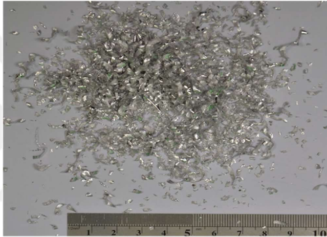
Figure 42. Chip forms of AZ91 alloy at conditions: V_c :640 m/min, V_f :0.95 mm/min
