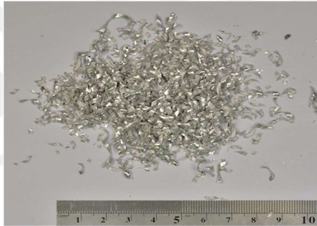
Figure 45. Chip forms of AZ91/2.5 wt.% rCF composite at conditions: V_c :640 m/min, V_f :0.65 mm/min
