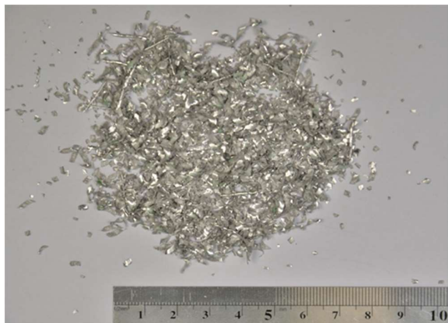
Figure 46. Chip forms of AZ91/5 wt.% rCF composite at conditions: V_c :480 m/min, V_f :0.95 mm/min
