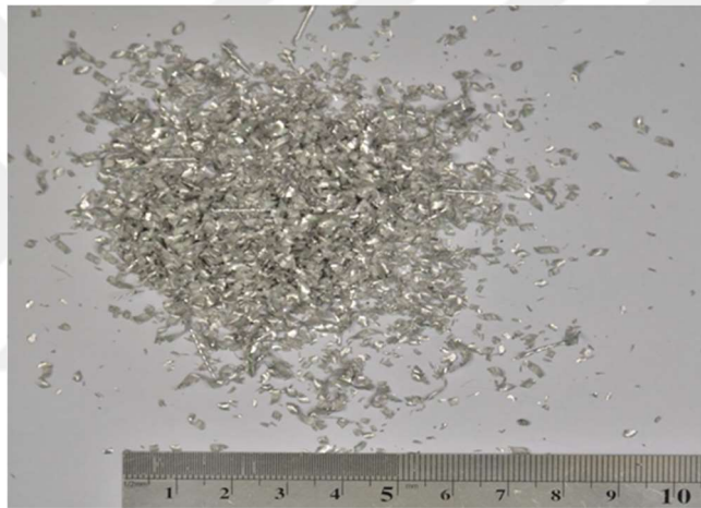
Figure 48. Chip forms of AZ91/5 wt.% rCF composite at conditions: V_c :640 m/min, V_f :0.80 mm/min
