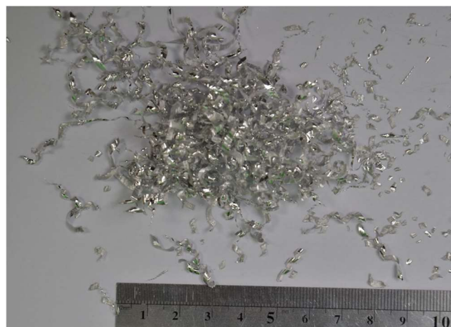
Figure 40. Chip forms of AZ91 alloy at conditions: V_c :480 m/min, V_f :0.65 mm/min
