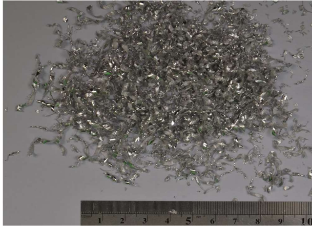
Figure 41. Chip forms of AZ91 alloy at conditions: V_c :560 m/min, V_f :0.80 mm/min
