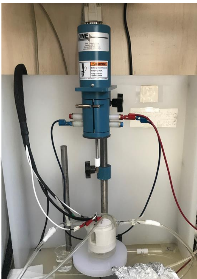
Figure 3.4. A potentiostat is connected to three electrodes in a cyclic voltammetry setup: the working electrode (WE), the counter electrode (CE), and the reference electrode (RE). In a jacketed pot, the electrode tips were immersed in electrolyte solution.
