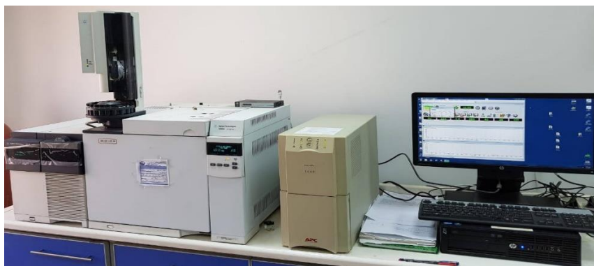
Figure 3.1 GC MASS device. Analytical Column: Agilent HP-5ms Ultra lent (30 m length x 250 \mu\text{m} diameter x 0.25 \mu\text{m} inside diameter), Injection volume 1 \mu\text{l} and Pressure 11.933 psi; GC Inlet Line Temperature: 250 ^{\circ}\text{C} ; Aux heaters Temperature 300 ^{\circ}\text{C} ; Carrier Gas: He 99.99%; Injector Temperature: 250 ^{\circ}\text{C} Scan Range: m/z 25-1000; Injection Type: Split less; Oven Program: Temperature; Ramp 1: 60 ^{\circ}\text{C} hold to 3 min.; Ramp 2: 60 ^{\circ}\text{C} to 180 ^{\circ}\text{C} 7 ^{\circ}\text{C}/\text{min} ; Ramp 3: 180 ^{\circ}\text{C} to 280 ^{\circ}\text{C} 8 ^{\circ}\text{C}/\text{min} ; Ramp 4: 280 ^{\circ}\text{C} hold to 3 min
