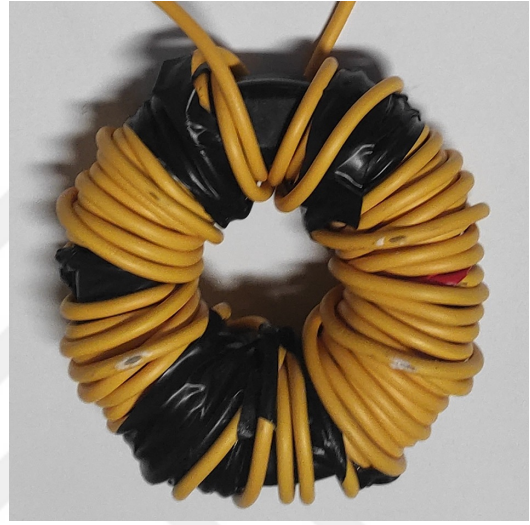
(b) Inductor with thick insulation
