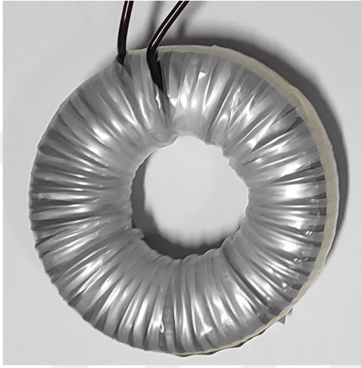
(a) Inductor with thin insulation
