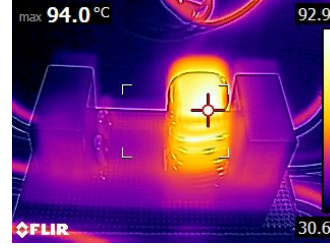
(b) Out-of-phase switching, 21.2 A, after 6 minutes
