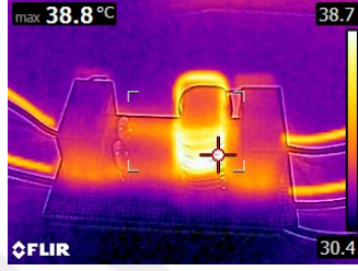
(c) In-phase switching, 16.9 A, after 10 minutes
