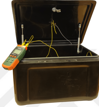
Figure 4.16: Calorimeter setup to measure losses of the components
