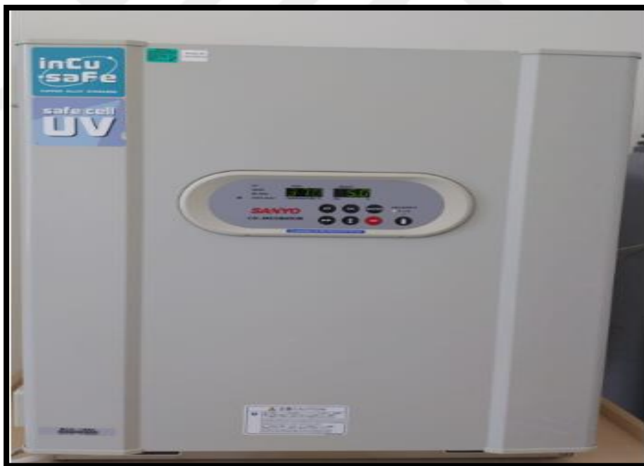
Figure 3.2. CO 2 Incubator 5% of atmospheric carbon dioxide in 95% humidified at 37°C
