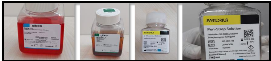
Figure 3.8. Dulbecco's Modified Eagle Medium (DMEM) with supplementary (FBS, L glutamine, penicillin-streptomycin solution).
