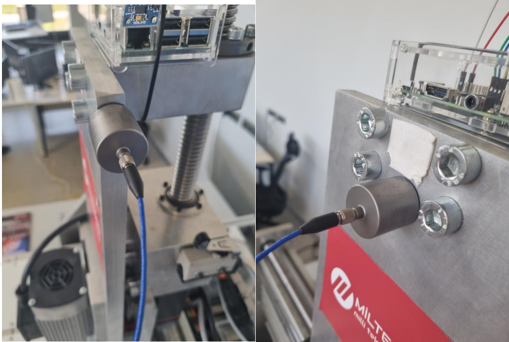
Figure 21 Piezo electric sensor placed on X and Y axes respectively.
