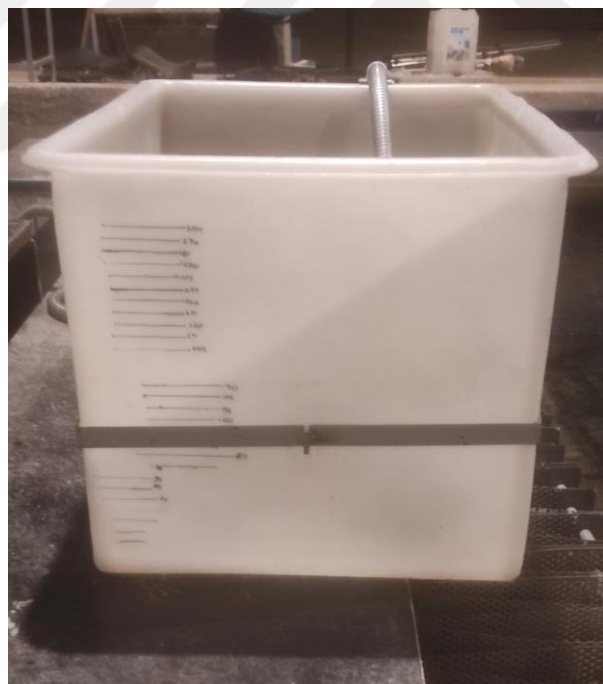
Figure 3.7 Overtopping collection tank
