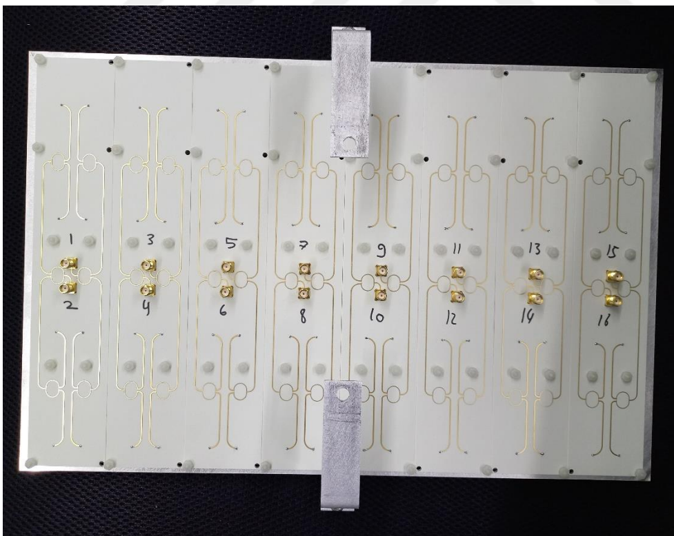
Figure 4.22. Bottom view of prototype antenna array
