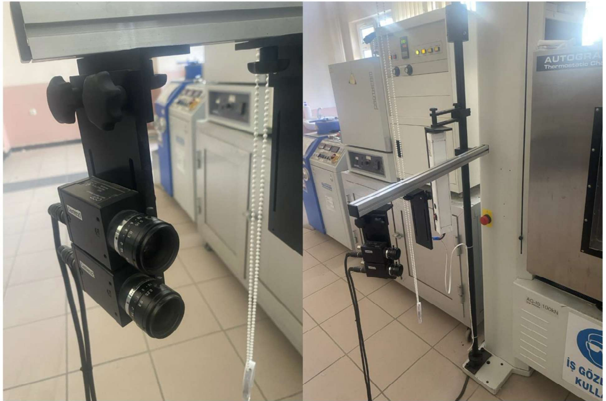
Figure 3.13 High-Definition Cameras integrated into Shimadzu software TRAPEZIUM
