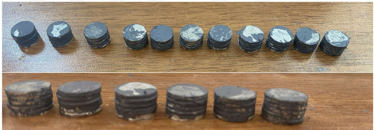
Figure 3.11 Prepared disc compression specimens, (dry graphite lubricated and in 5 stack)
