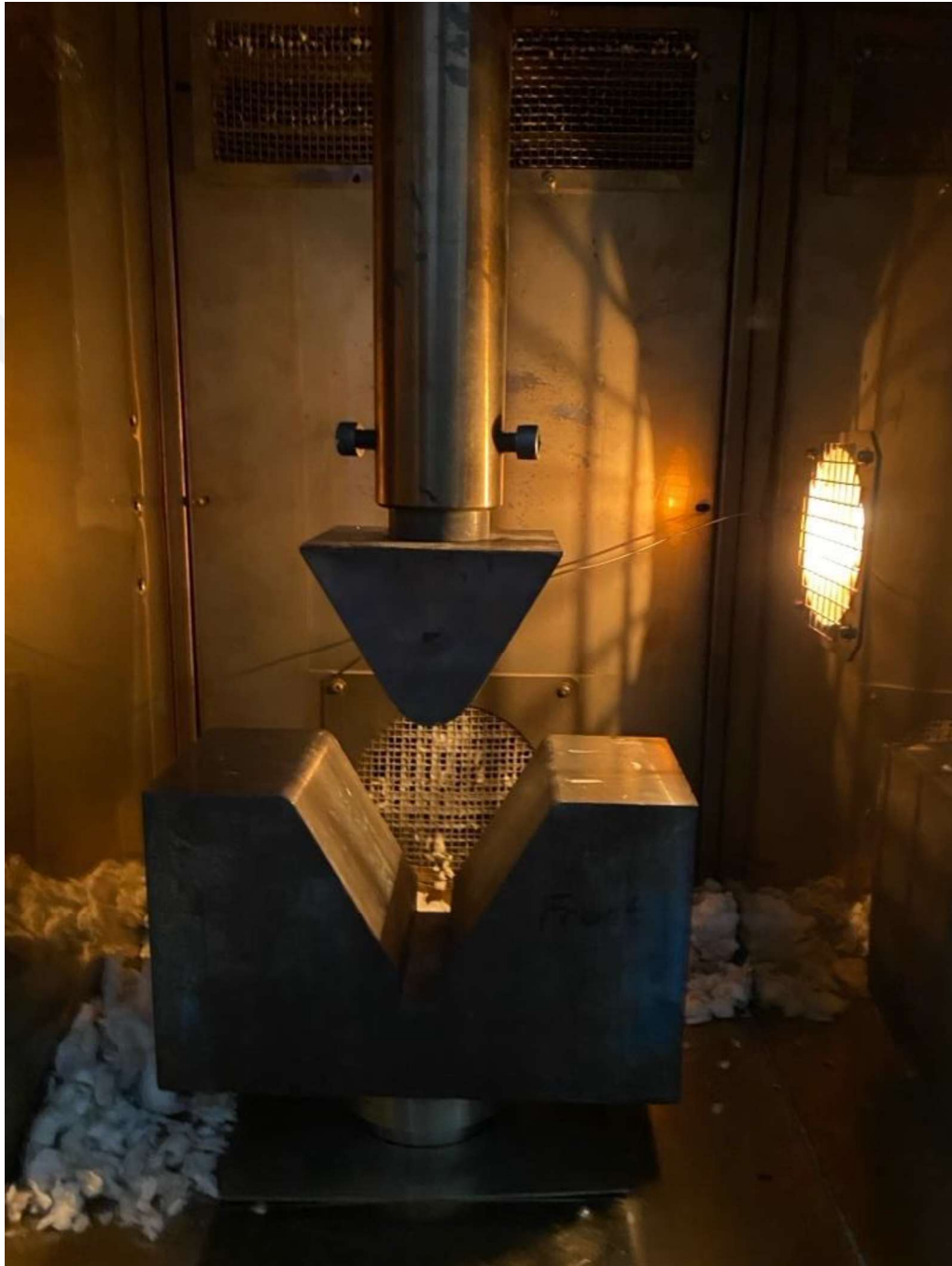
Figure 3.3 V Bending test apparatus with 60° punch and the die used in procedure, inside the thermostatic chamber
