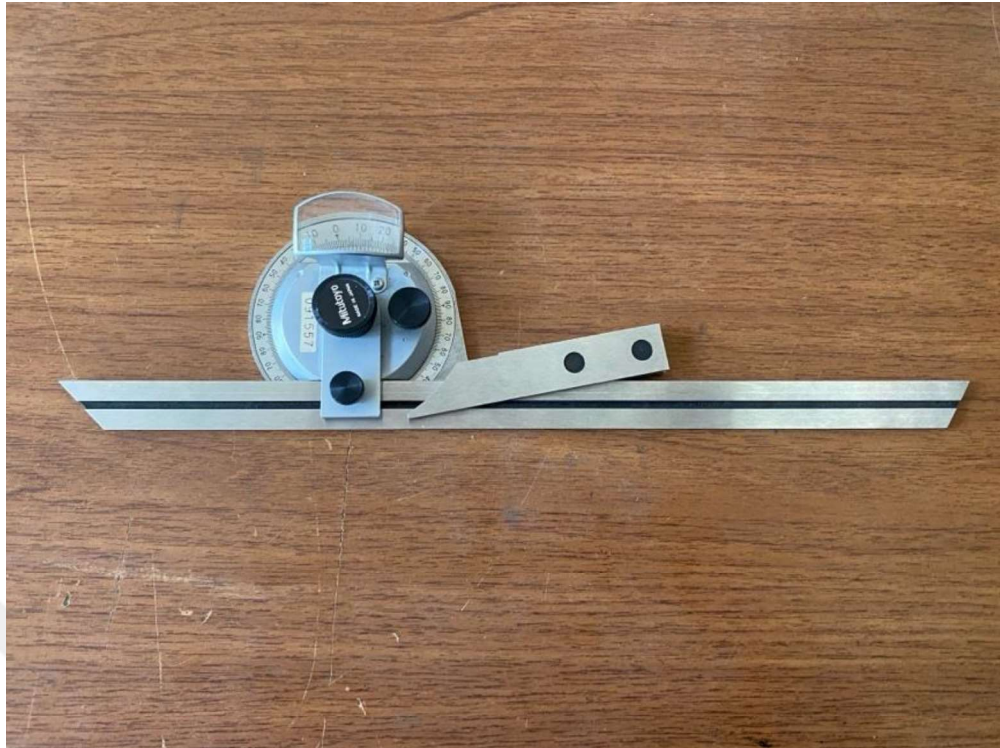
Figure 3.7 Mitutoyo 187-906 Universal Protractor used in springback angle measurements
