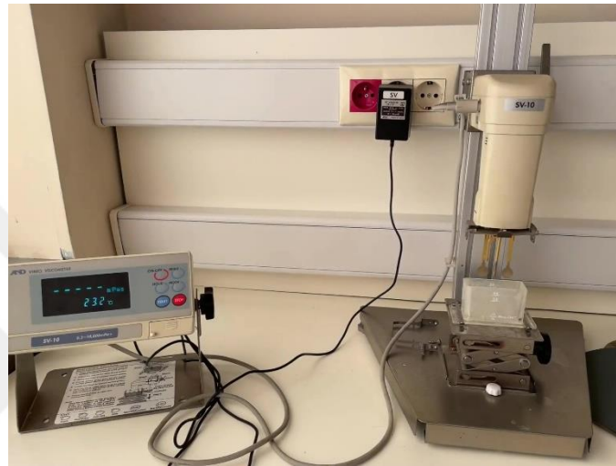
Figure 3.2: Viscosity measurement set-up for identifying viscosity of chitosan solutions used in the experimental work.
