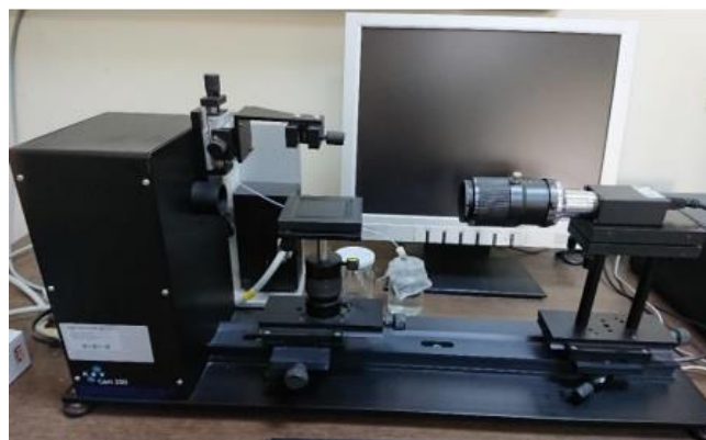
Figure 3.4: Chitosan polymer solution surface tension analysis.
