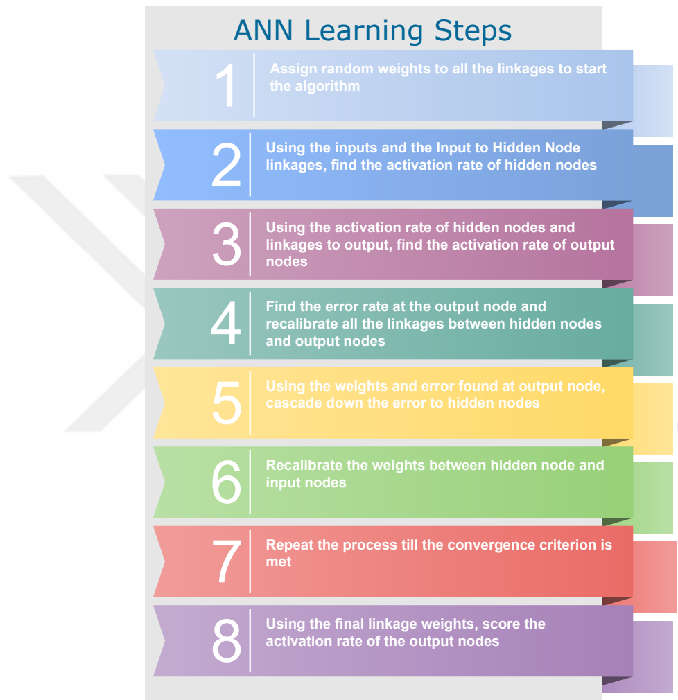
Figure 2.10 An illustration of the various steps involved in the learning process of an ANN, including the initialization of weights, the forward propagation of inputs, the calculation of errors, and the adjustment of weights to minimize errors [12]
