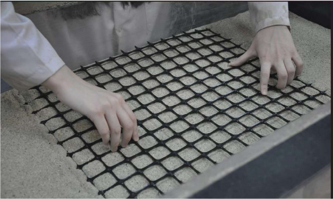
Figure 3.21. Placing the geogrid reinforcement.
