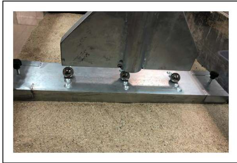
Figure 3.6. Placement of marbles with hexagonal loading plate.
