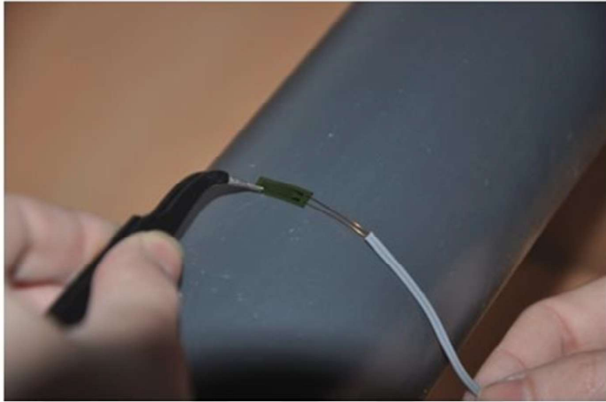
Figure 3.19. Strain gauge placement on the pipe.
