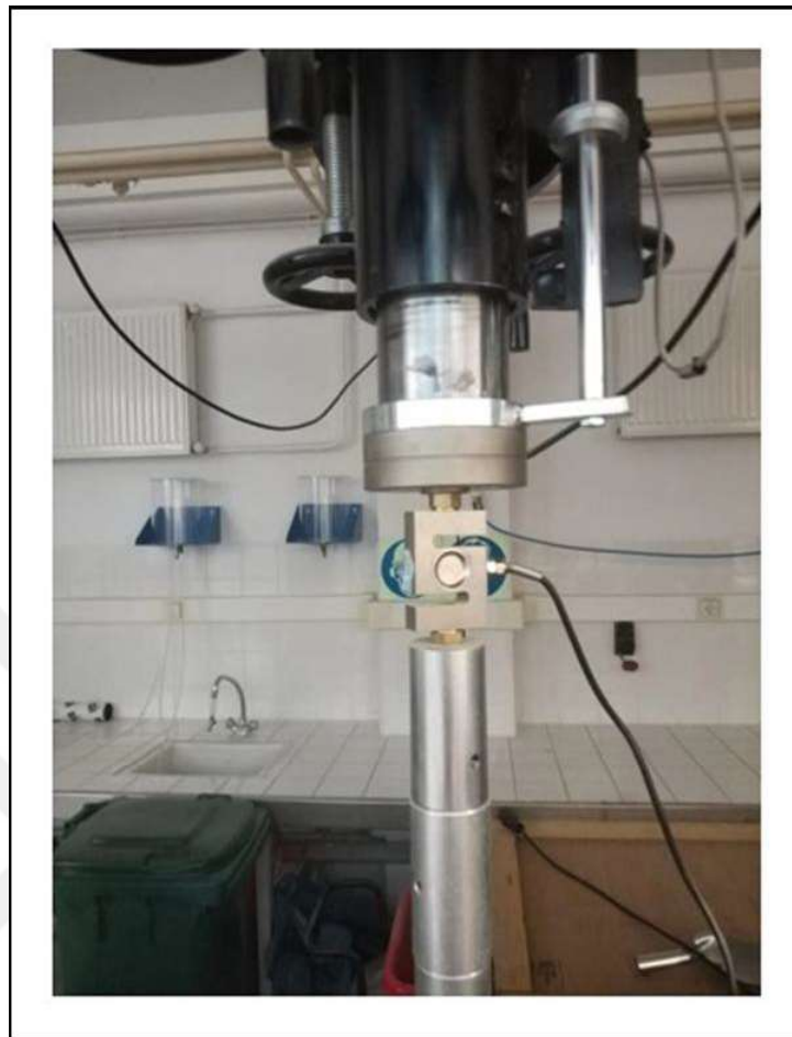
Figure 3.9. 500 kg S-type load cell used in the experiments.
