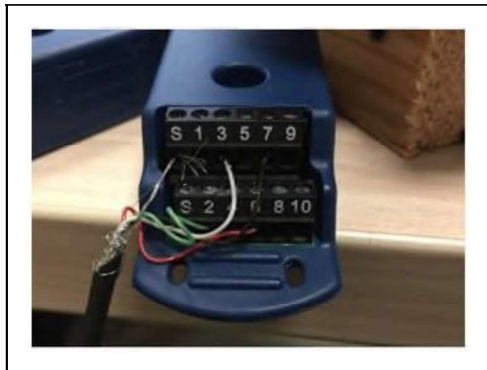
Figure 3.15. NI-9949 terminal adapter
