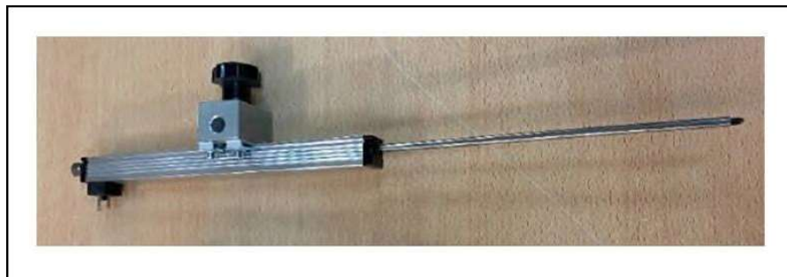
Figure 3.8. LVDT transducers used in the experiments.
