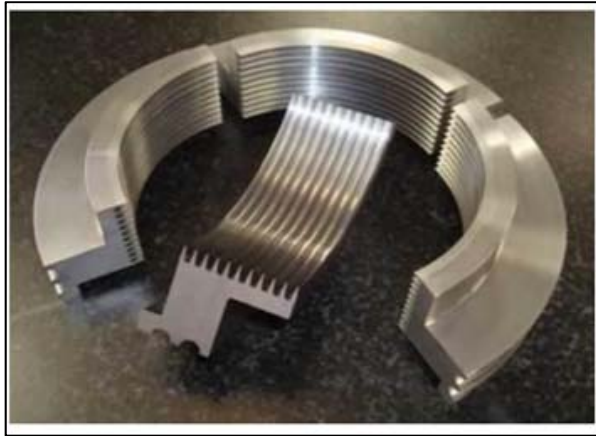
Figure 1.7: Straight Through Labyrinth Seal
