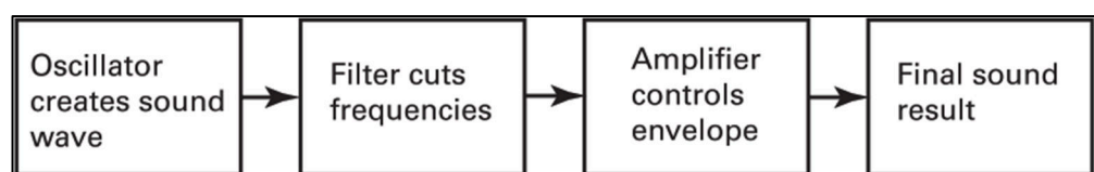
Figure 1. Subtractive synthesis of sound generation (Collins, 2008)
