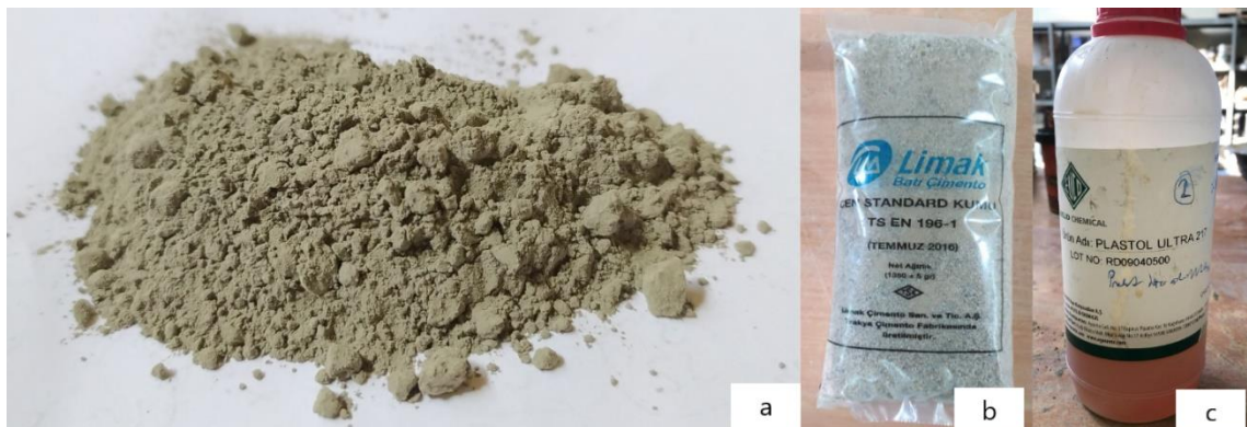
Figure 3.1 a) Portland cement (OPC) CEM I 42.5 R, b) Standard sand, c) Polycarboxylate Superplasticizer (SP)
