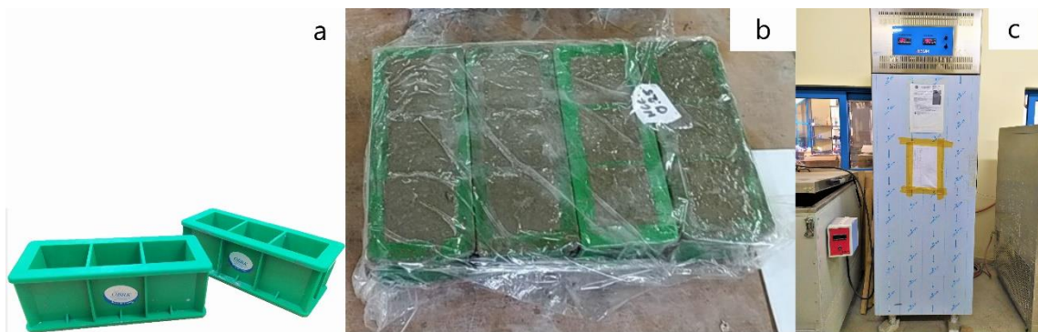
Figure 3.10 a) Plastic mold (50 X 50 X 50 mm), b) molded mortars samples cover by cling film sheet, c) moist cabinet
