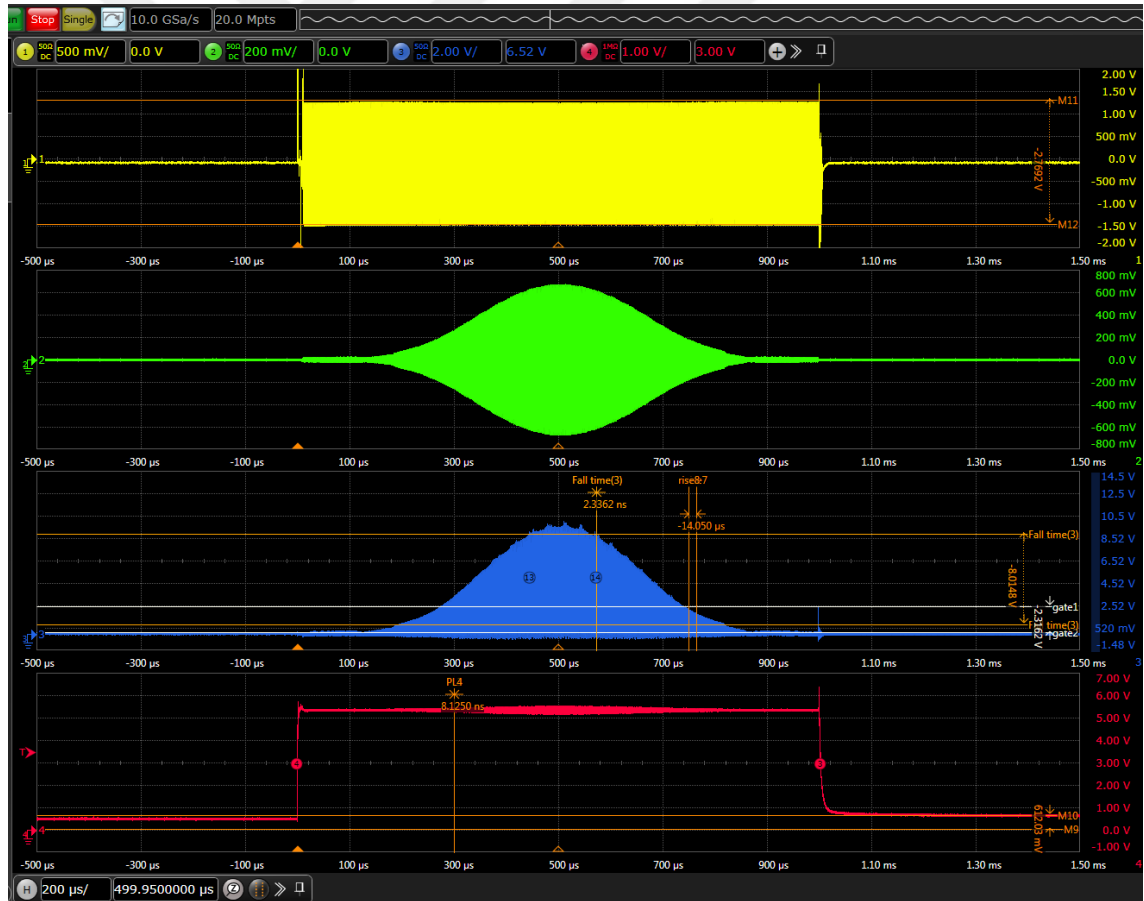
Figure 4.15: RF gating method signals for a 1.25ms RF pulse from top to bottom: (yellow) 3.2x scaled version of logic buffer output signal, (green) output RF pulse sensed by the pickup coil, (blue) V_{ds} voltage of the Class-E amplifier, (red) Output voltage level feeding the logic buffer
