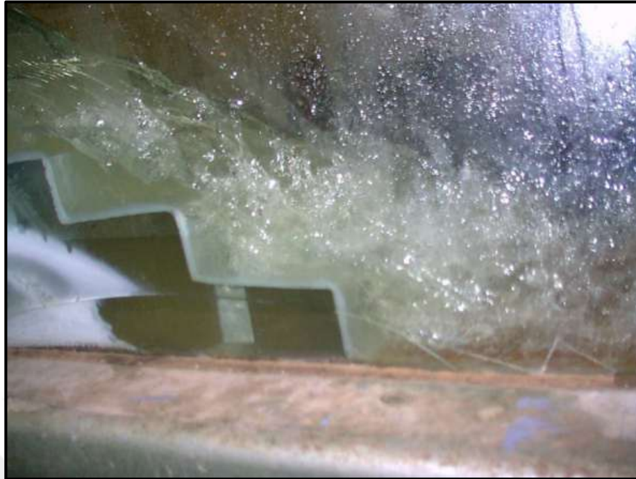
Figure 2.1 Turbulent flow and energy dissipation (Salmasi and Samadi 2018)
