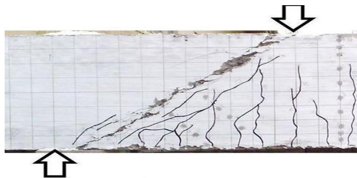
Figure 2.16 Diagonal Splitting failure, by Ismail, 2016
