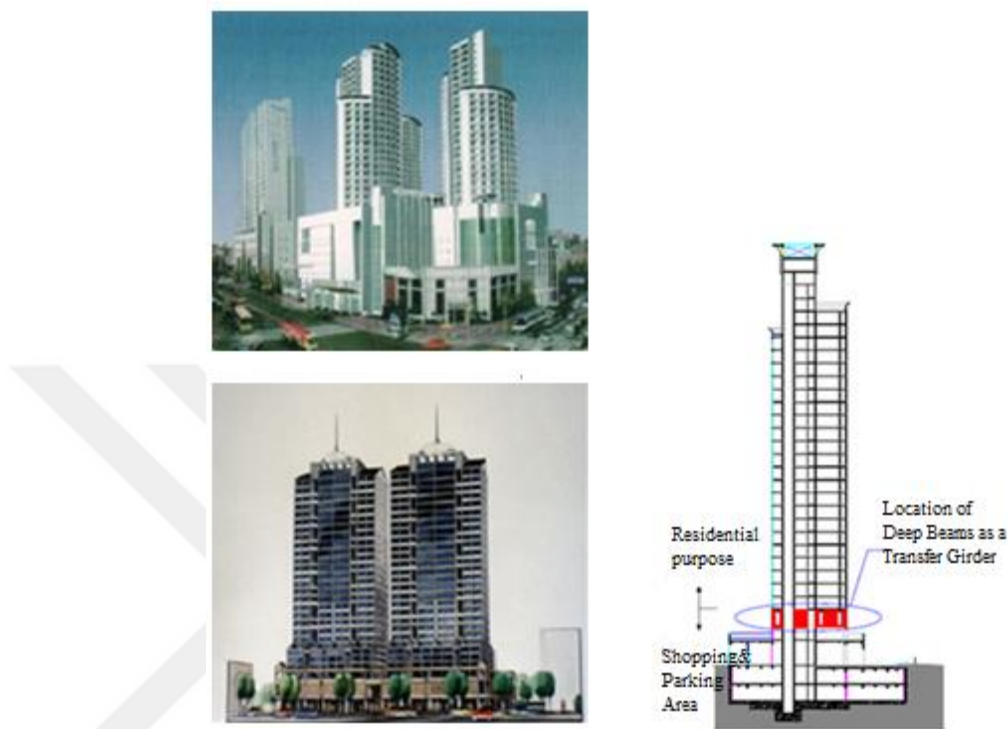
Figure 2.1 Deep beams location and uses (Khair, 2005)
