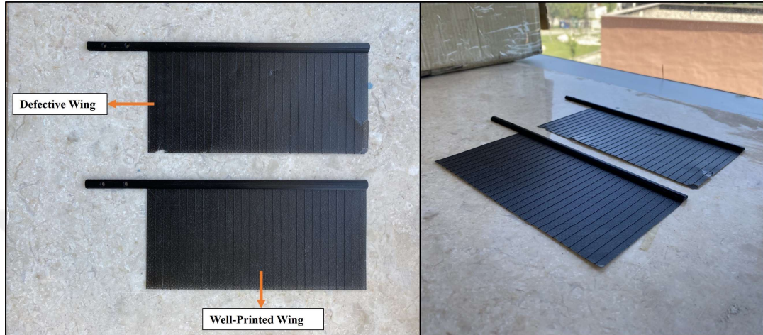
Figure 3.8. Defective wing and well-printed wing
