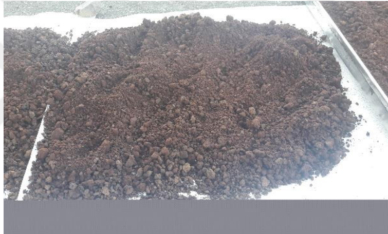
Figure 4.1 Air-dried drinking water treatment sludge (Personal archive, 2019)
