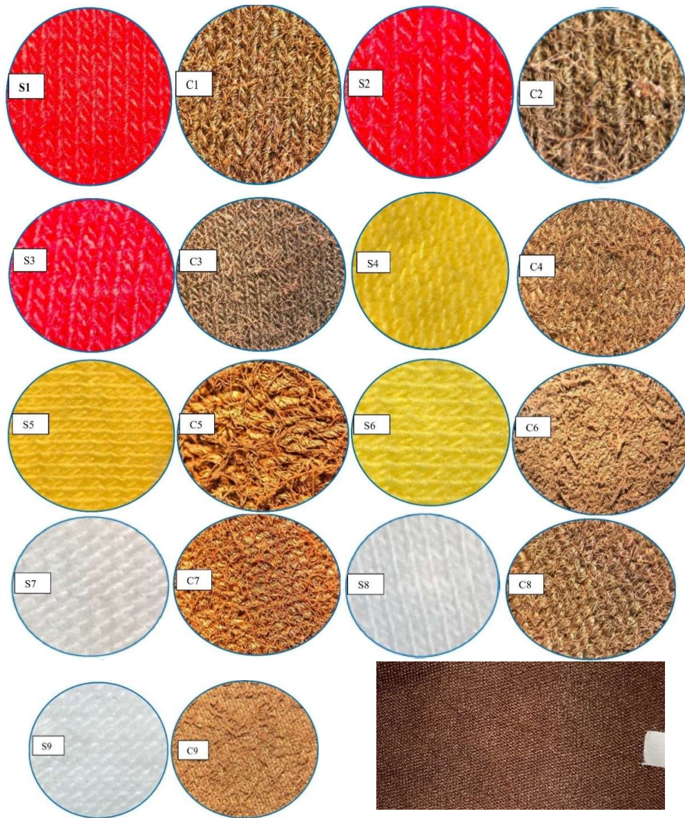
Figure 4.1 : Microscopic morphology of all the uncoated and coated Knitted cotton fabric.
