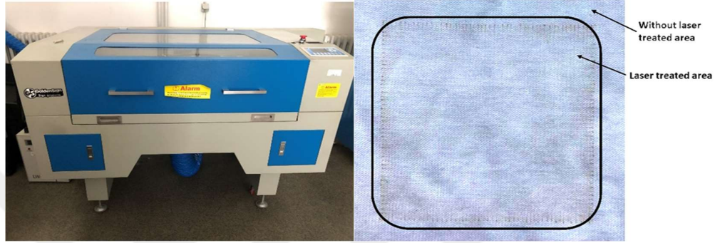
Figure 3.4 : Golden sign laser cutting machine GS1490 and laser-treated area.
