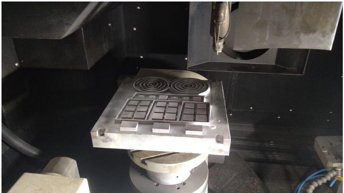
Figure 4.14 Synova MicroJet Laser system and test part
