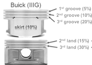
Figure 2.1. Engine piston groove and lands.
