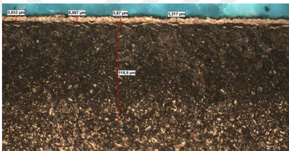
Figure 4.1 1.2344 tool steel nitriding layer before annealing(preheating) by optical microscope 500x
