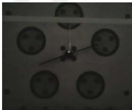
Figure 3.6 Nitrided specimens are suspended in inert gas furnace
