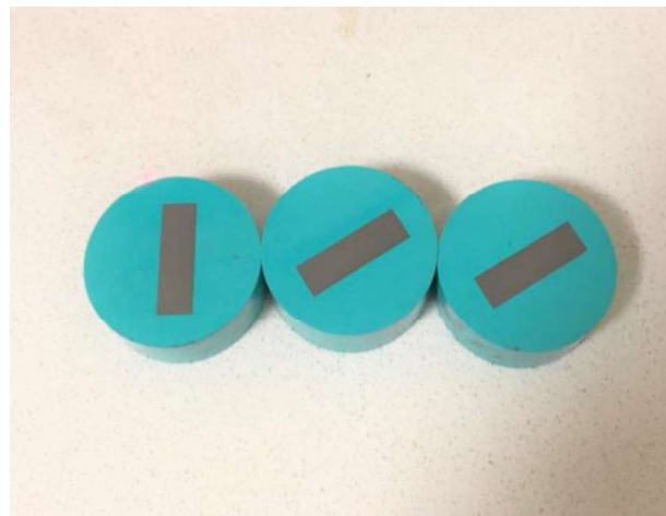
Figure 3.8 At 535 °C 6 hours nitrided and mounted 1.2344 hot work steel specimens
