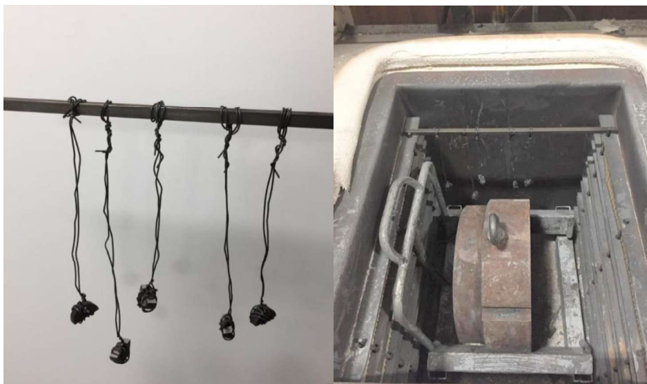
Figure 3.5 Nitrided specimens are suspended in air furnace
