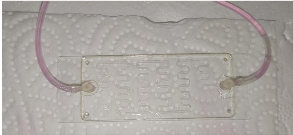
Figure 4.2 Leakage test of microfluidic chip
