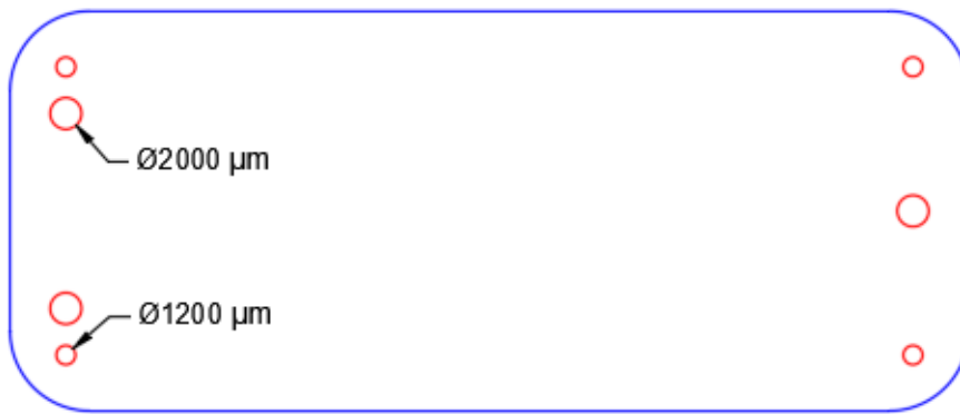
Figure 3.4 CAD design of top layer (one inlet-one outlet)
