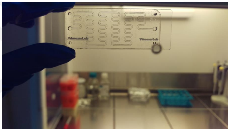
Figure 3.6 Assembled microfluidic chip (one inlet-one outlet)
