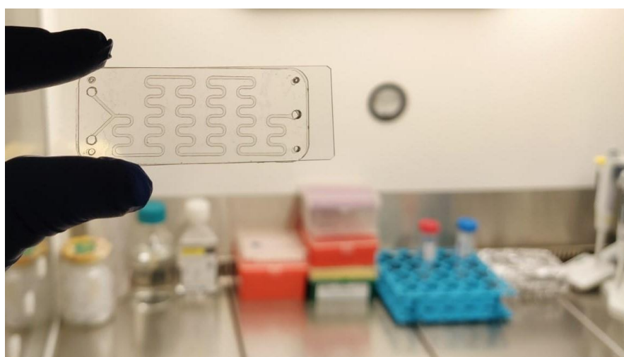
Figure 3.7 Assembled microfluidic chip (two inlets-one outlet)
