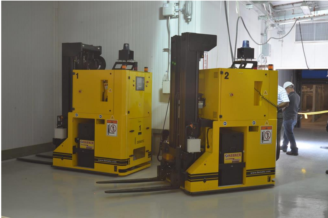
Figure 1. Figure of an AGV
