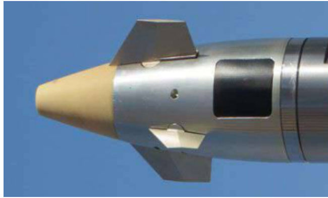
Figure 1.2: An Example Design Which Uses Movable Aerodynamic Surfaces
