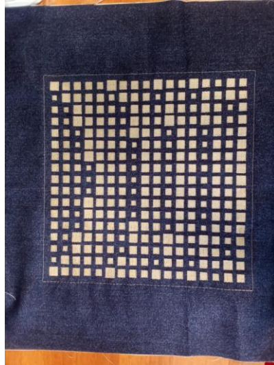
Figure 6.3. Fabricated offset feed reflectarray.
