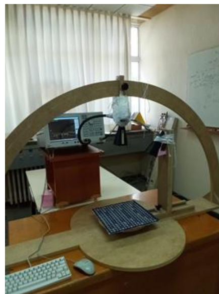
Figure 6.8. Measurement setup for offset feed configuration.
