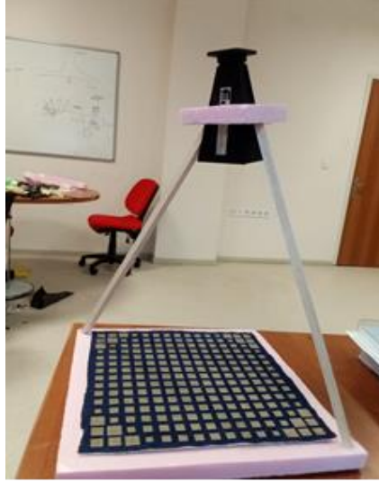
Figure 6.5. Measurement setup for center feed configuration.
