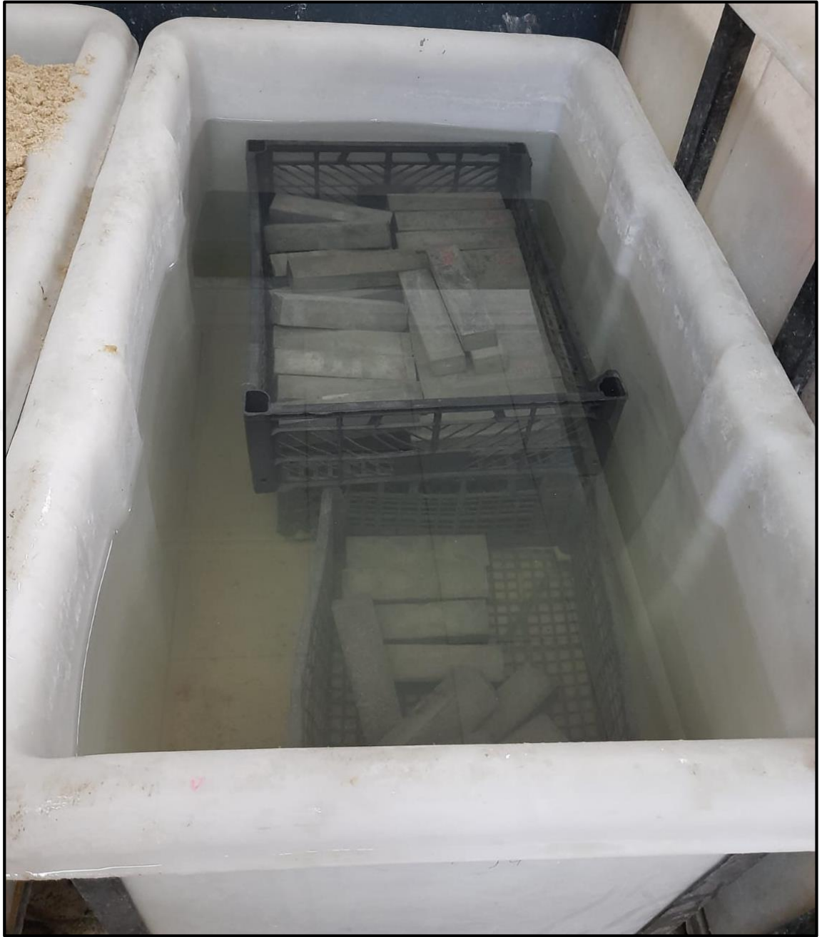
Figure 3.11 Room temperature curing basin
