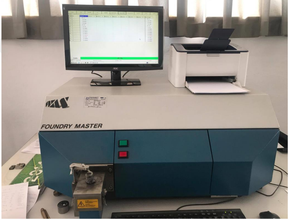
Şekil 5.20 : WAS Foundry Master kimyasal analiz spektrometresi.
