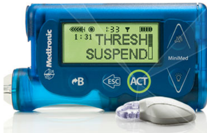
Figure 2.3 Insulin pump with continuous glucose measurement system [26]
