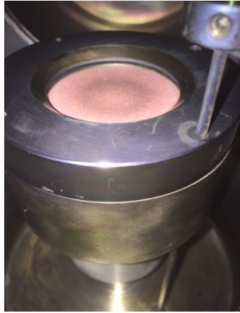
Figure 3.2. Bi2212 target used in our RF magnetron sputtering system.
