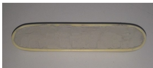
Figure 5.1. The obtained homogenous powder mixture and alumina crucible.
