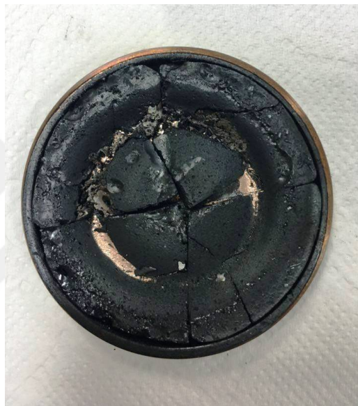
Figure 5.7. Photograph of the prepared Bi2212 target combined in a copper metal container after deposition processes.
