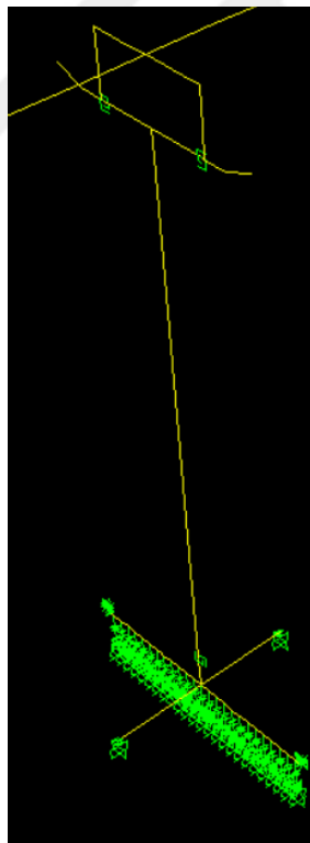
Figure 25. Takeda Link Located on the Cap Beam and Hammerhead Pier
