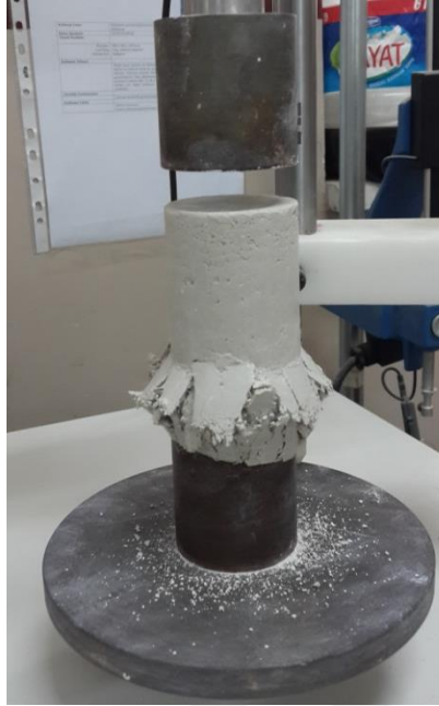
Figure 4.9. A fractured lime stabilized specimen containing polypropylene fiber (PF) after unconfined compression test
