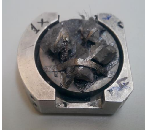
Figure 4.13. Specimens on the brass plate with a double sided adhesive carbon tapes
