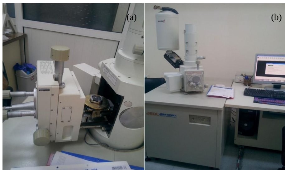
Figure 4.15. Image of a) placing and b) analyzing gold-plated specimens in SEM device
