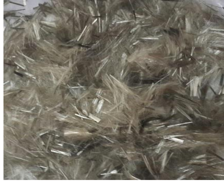
Figure 3.5. Image of crumbled BF
