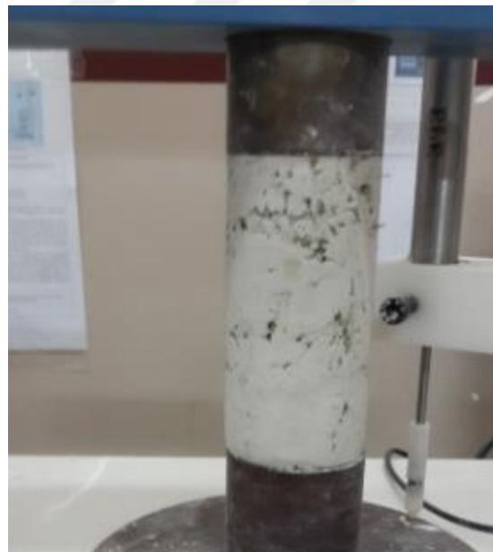
Figure 4.5. Application of unconfined compression test to the specimen containing basalt fiber (BF)
