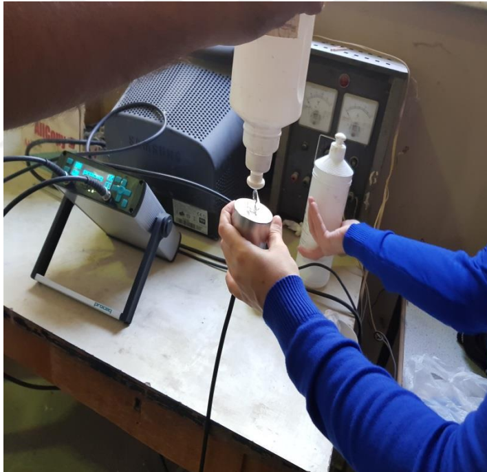
Figure 4.24. Application of ultrasound gel to the transducer
