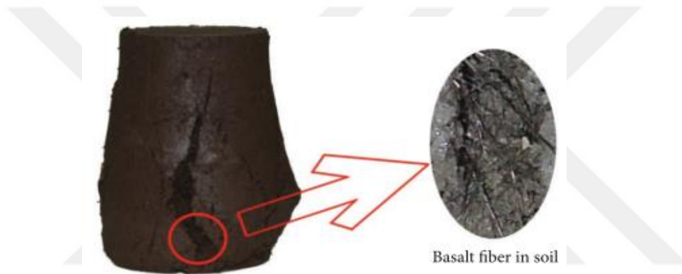
Figure 2.5. Failure form of basalt fiber amended soil specimen (Gao et al., 2015)
