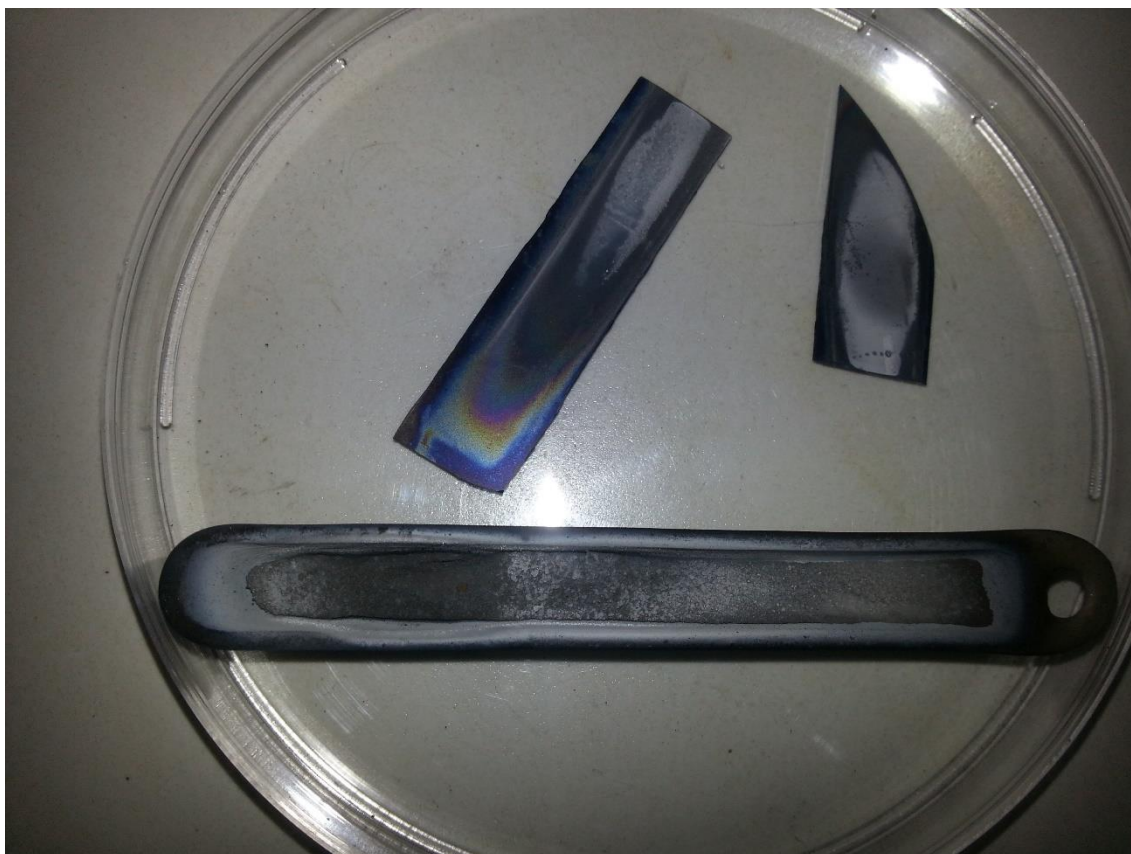
Figure 6. 3. BNNT production at 900 °C with NaFeO 2
