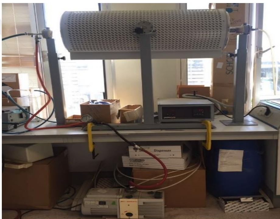
Figure 3. 1: Experimental Thermal CVD setup
