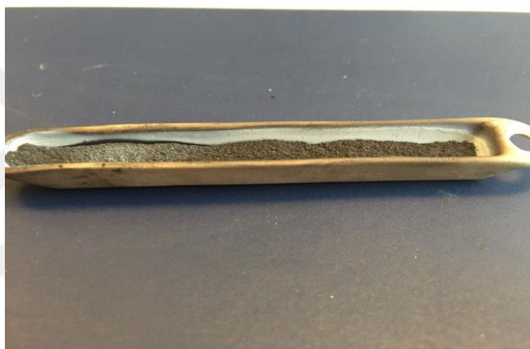
Figure 5. 3: As synthesized BNNTs on the substrates A) Ceramic substrate (bottom of the empty crucible, which was cut before and placed on the top of the combustion boat) B) walls of combustion boat
