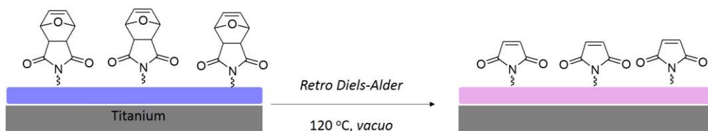
Figure 8.6. Removal of furan groups via retro Diels-Alder reaction.
