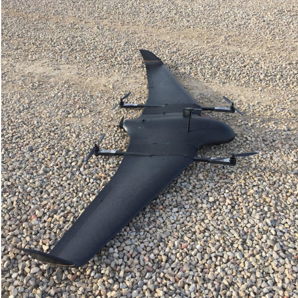
Şekil 1.5 Deltaquad VTOL İHA (Vertical Technologies, 2018)
