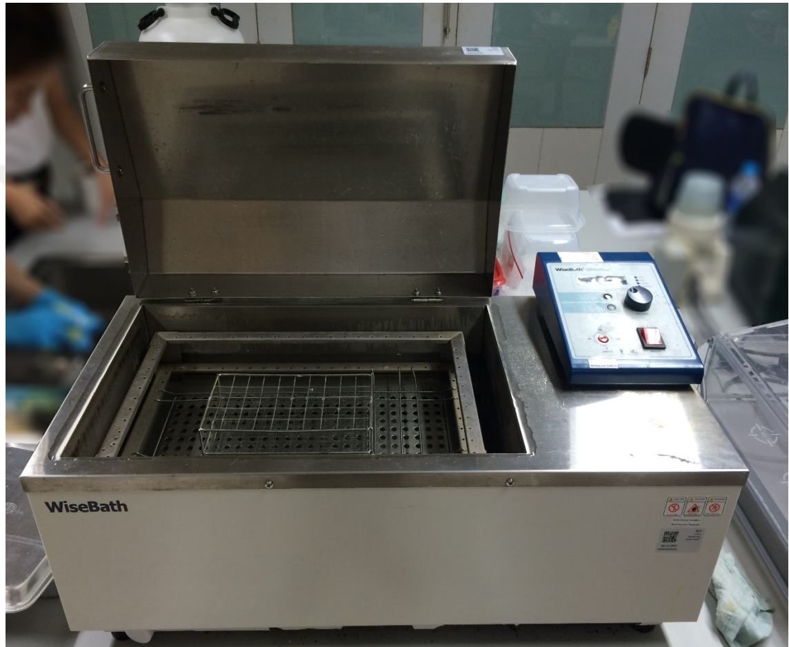
Figure 3.6 Laboratory water bath, A water bath operating at 72°C
