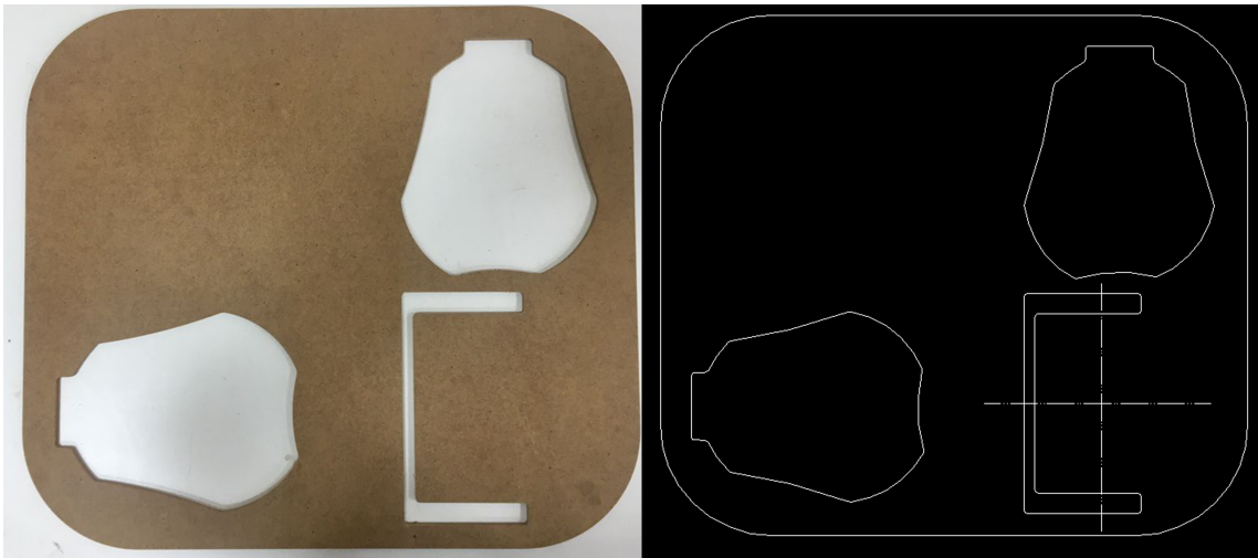
Figure 4.3. Reference settlement plate and its 2D design
