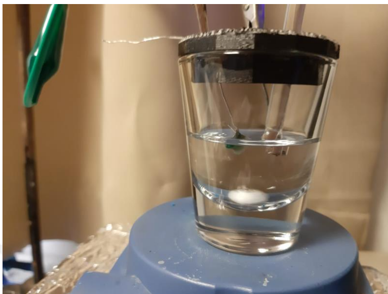
Figure 31. The three-electrode setup for the electrocatalytic water oxidation, in which the cobalt PBA is the working electrode connected to Pt cathode as the counter electrode with an external electric wire, and Ag/AgCl as the reference electrode, all of which immersed in the 0.1 M phosphate buffer solution with pH = 7.
